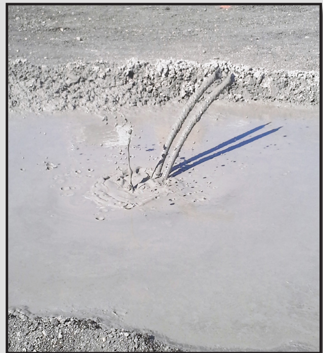
Figure 2. Shallow gas bubbling up through mud in a drillhole at the geothermal well field site near Hillsboro. Several other drillholes in the well field exhibited the same behavior for an approximate two-week period but dissipated shortly thereafter.
