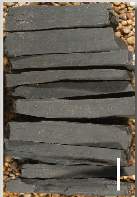
Figure 5. Photograph of a representative core sample showing the source beds in the Icebox Formation (SESW Sec. 1, T152N, R90W, EOG Resources, Inc. – Shell Creek #1-01; Depth 13,143.5 – ft.). The Icebox consists of a gray-green massive to finely laminated, fissile, organically-lean shale that reaches a maximum thickness of 49 m (160 ft.). Scale bar shown in white is 1 inch.
