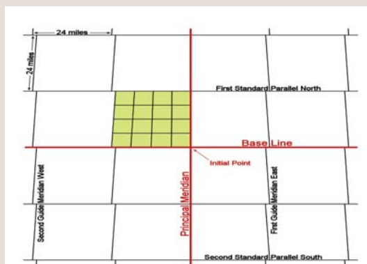
Figure 4. Survey of quadrangles (white squares) and their division into townships (green squares).
