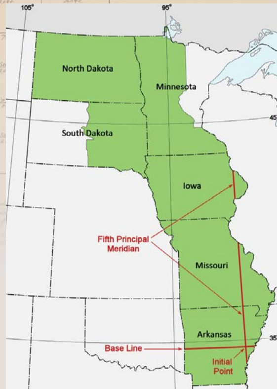
Figure 2. The Fifth Principal Meridian governs the surveys of all or part of six states (shown in green).
