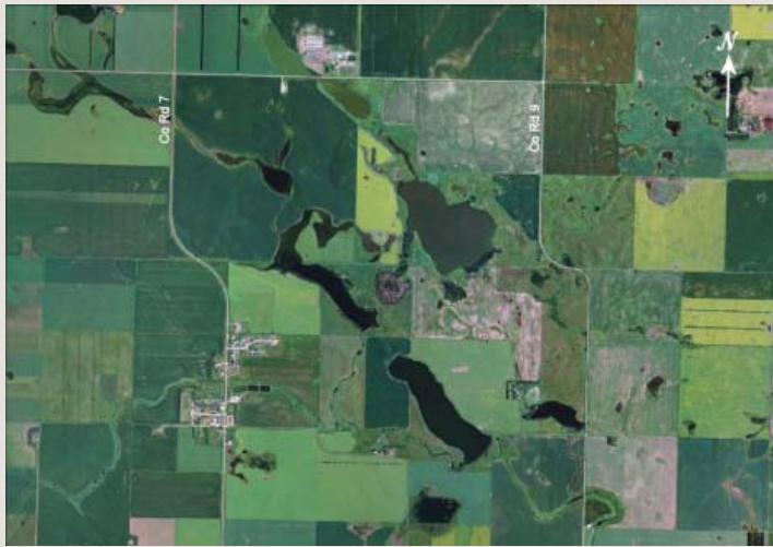
Figure 8. McLean County Roads 7 and 9 turn abruptly west where they meet the Twelfth Standard Parallel between Townships 148 and 149 North before resuming their northward track near the community of White Shield. The Twelfth Standard Parallel is a correction line that allows surveyors to compensate for the earth's curvature by resetting the six-mile interval between range lines. The adjustment causes a slight westward shift in the rows of townships north of the line.
