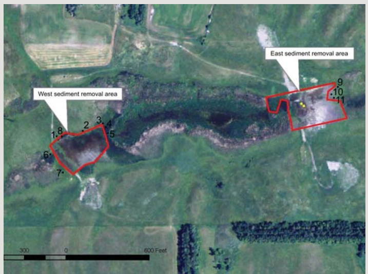
Figure 2. Aerial photograph of the Tolna Coulee study site. The areas outlined in red are where the City of Devils Lake removed sediment down to an elevation of 1,458 feet; the 1997 trenches are yellow squares, and the 2011 core sites are shown as numbered black squares.
