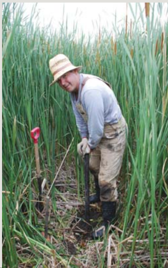
Figure 1. Fred Anderson (NDGS) pushing a core barrel (with an interior plastic sleeve) through organic-rich sediment in the Tolna Coulee.
