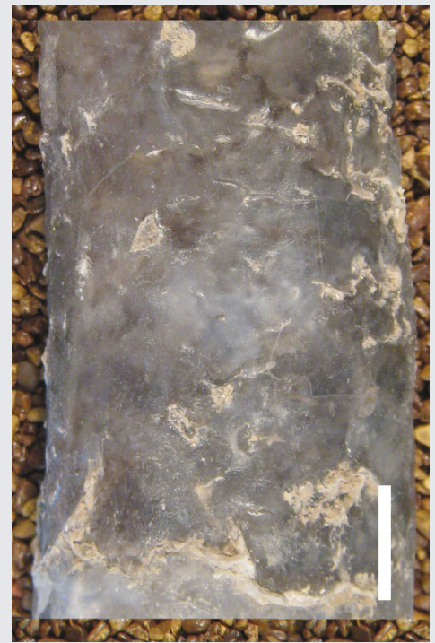
Figure 3. Core photograph of the Prairie salt from the Prairie Formation from the Pan American Petroleum Corp. - #1 Clifford Marmon (API #33-105-00667-0000; Depth – 11452 ft.; SWSW Sec. 2, T154N, R95W). Note the silt and clay stringers throughout the halite beds. White scale bar = 1 inch.
