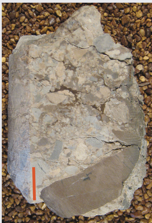
Figure 5. Core photograph of a polymictic breccia consisting of multiple lithologic clasts floating in a mudstone matrix from the Prairie section in the California Company - #1 Blanche Thompson (API #33-009-00002-0000; Depth: 6345 ft.; SWSE Sec. 31, T160N, R81W). The breccia is the result of the dissolution and removal of the Prairie salt and the subsequent collapse of the overlying strata.
