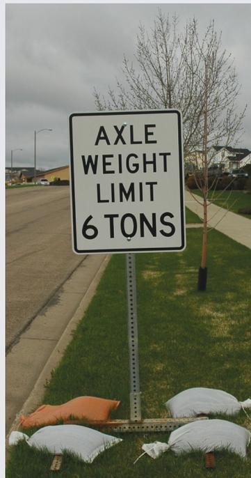
**Figure 7.** Load restrictions are imposed to prevent damage to roads weakened by meltwater saturation during the spring thaw. Photo by Lorraine Manz.
