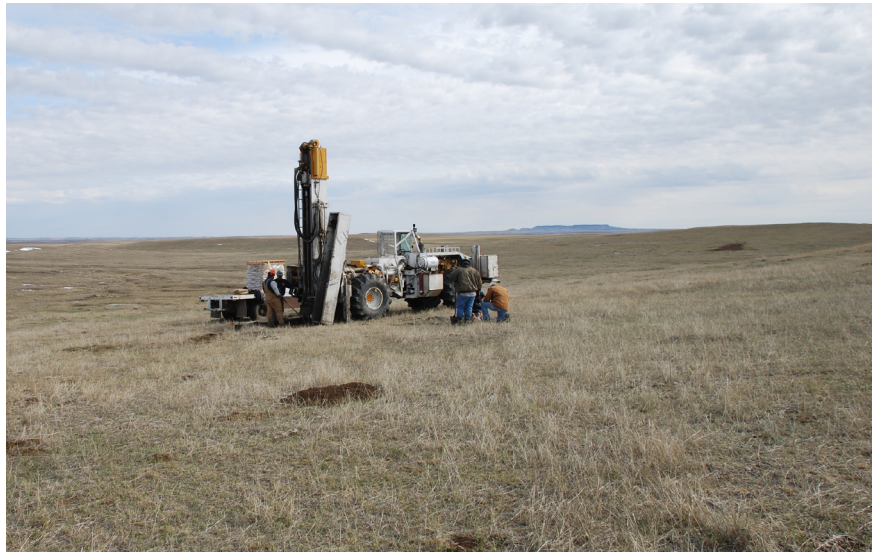
Figure 1. Geologists collect lignite samples for germanium analysis from a hole drilled near the old Church or Fritz mine in southern Billings County.
