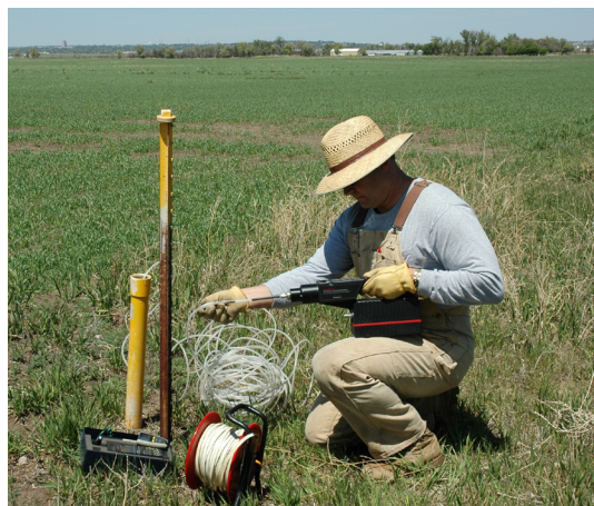
Survey geologist Fred Anderson field screening for shallow gas (methane) in shallow ground-water observation wells in southern Burleigh County during the 2008 field season. Recent results and highlights from this investigation were presented this fall at the 2008 Rocky Mountain Unconventional Gas Conference in Rapid City, South Dakota.
