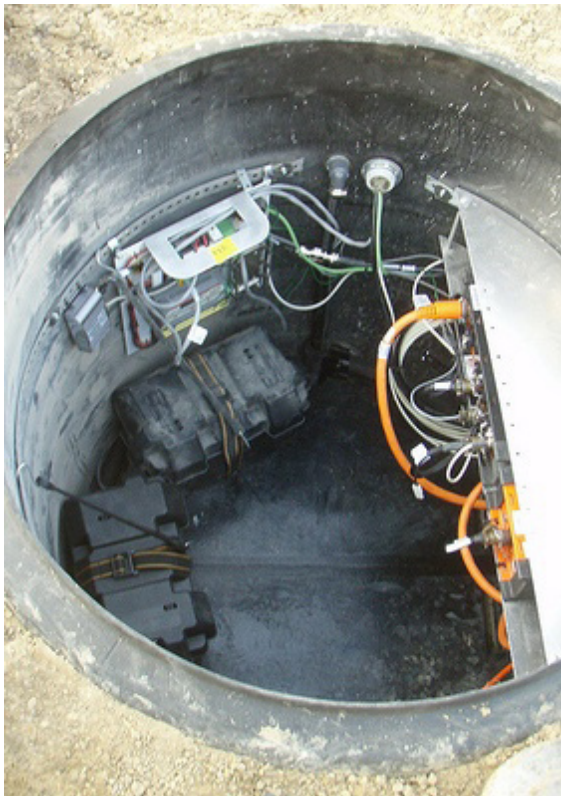
Figure 5. On the left: instrumentation and auxiliary sensors installed in the upper vault section of the Maddock station. On the right: seismometer installed on a concrete pad at a depth of about six feet in the lower vault section of the Maddock station. Images courtesy of EarthScope, 2008.
