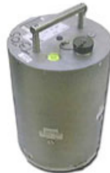
Figure 7. Guralp CMG3T broadband seismometer. This more durable type of seismic monitoring instrument has been installed at the Westby station as part of the Transportable Array (TA) network and is also currently operational. Image courtesy of EarthScope, 2008.
