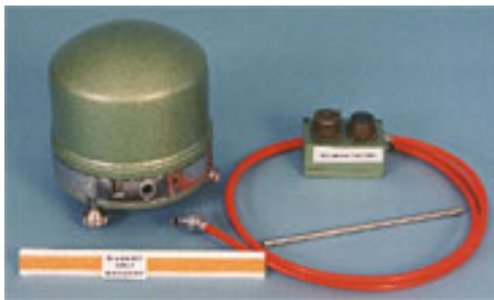
Figure 6. Streckeisen STS-2 three-component broadband seismometer. This type of seismic monitoring instrument has been installed at the Maddock USArray reference network station and is currently operational. Image courtesy of EarthScope, 2008.
