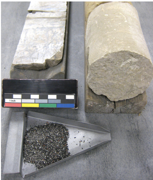
Figure 1. Core and samples (drill cuttings) laid out on a work table in the laboratory of the core library. The core on the left is a rocker core of limestone taken from the Mission Canyon Formation at a depth of 3,780 feet in Tom F. Marsh's Clark no. 1 well in Burleigh County. The whole core on the right is limestone taken from the Mission Canyon Formation at a depth of 3,400 feet in I.J. Wilhite's Jensen U.C.L.I. no. 1 well in Bottineau County. The drill cuttings in the sample pan in the foreground are shales and mudstones from the Bakken Formation at a depth of 10,220 to 10,230 feet in Terra Resources Kling no. 1-7 well in Dunn County. More than half of the core in the core library is whole core that will eventually be slabbed and photographed.
