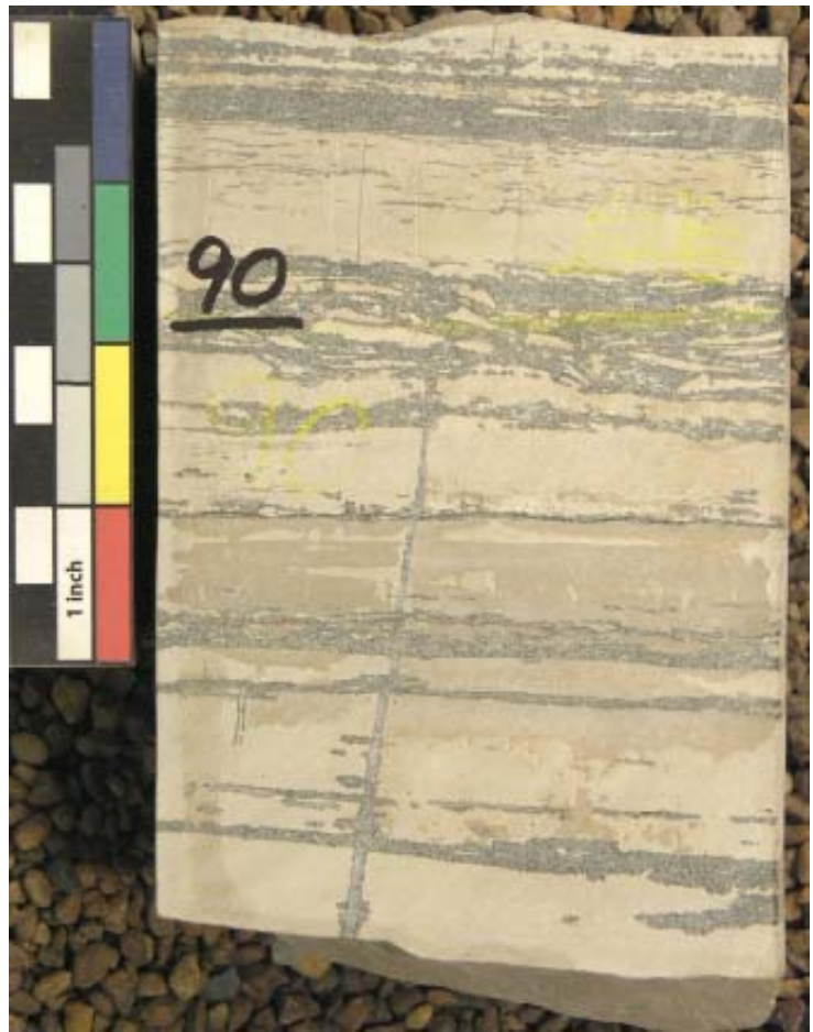
Figure 2 Core from the Three Forks Formation at a depth of 3,390 feet in the Daniel Anderson #1 drilled in Rolette County (NE SE sec. 17, T.160N., R.73W.). Note the mineralized (in-filled) vertical fracture and the flaser (wavy) bedding in this carbonate mudstone. The Three Forks is typically encountered at a depth of about 10,000 feet throughout much of the basin.
