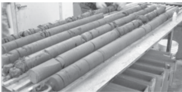
Figure 6. Sections of whole, intact core cut from the Niobrara Formation in south-central North Dakota being prepared and examined in the laboratory prior to sampling for detailed physical properties and geochemical analyses.
