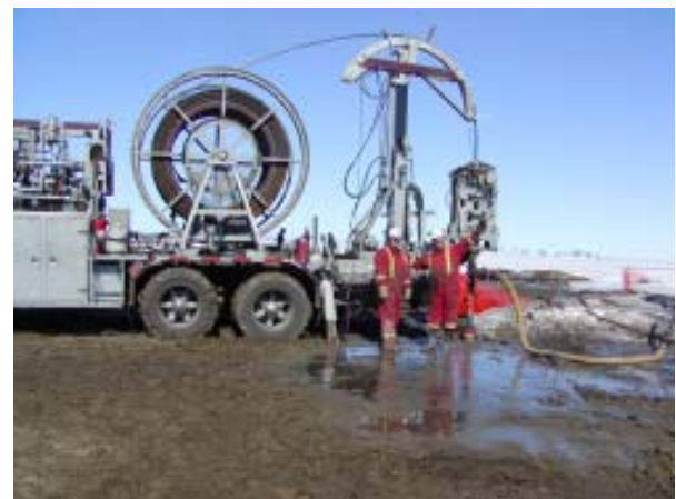
Figure 4. Stimulating the targeted zone of the Niobrara Formation in the Weiser well using a coiled-tube hydraulic fracturing rig.
