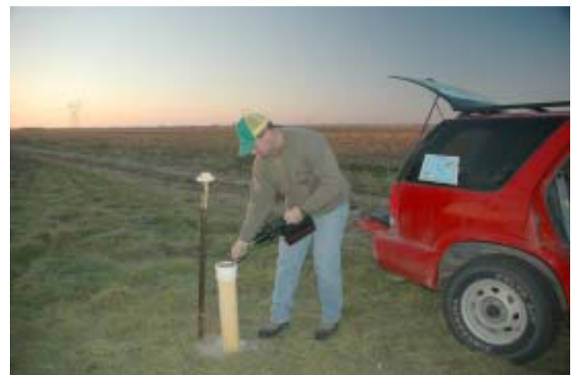
Figure 2. Field screening for shallow gas (methane) occurrence in a shallow ground-water observation well in Emmons County during the fall of 2006. The author is shown field screening a well with an FID at the observation well top of casing or TOC.
