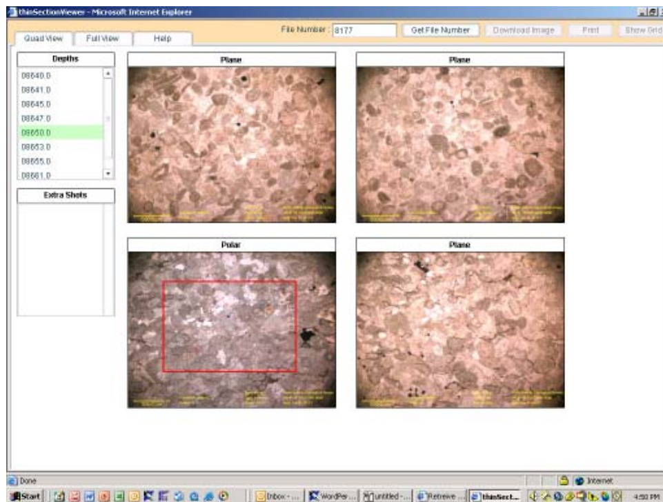
Figure 3. An example of a window that is visible when observing photomicrographs on the Oil and Gas subscription website. Approximately 80% of the thin section is displayed in the four quadrants. Each quadrant is photographed under plane and polarized light and the view can be changed by scrolling over the photographs. The area within the highlighted box will expand to fill the entire screen with the click of a mouse. These photomicrographs were taken at a power of 4x. This is a thin section of core from the Bakken Formation at a depth of 8,650 feet in the Dobrinski well no. 18-44 (NDIC permit no. 8177), Ward County, North Dakota.
