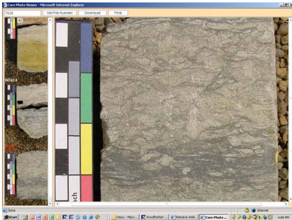
Figure 2. An example of a window that is visible when observing core photographs on the Oil and Gas subscription website. All core photos for a given well are placed in stratigraphic order along the left column where they can be scrolled through and a section of the core highlighted to generate the close-up photo of core in the window on the right. This is a photograph of a core of (bioturbated) burrowed sandstone from the Deadwood Formation (Cambrian\Ordovician). The core is from a depth of 10,342 feet, in the William Steckler well no. 1 (NDIC permit no. 7020), Grant County, North Dakota.
