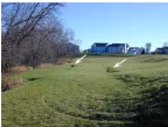
Figure 4. View to the south along the eastern bank of the Red River depicting earthflow, soil slumping, and bank failure near residential developments in north Fargo. Note the subvertical orientation of trees and presence of developing scarps in the foreground (Photo by Anderson).
