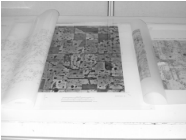
Compilation of a quarter-quad map from Renville County. The new orthophotoquad, which goes on the bottom, is shown in the middle of the photo; the old, half-toned orthophoto has been peeled to the right, and the clear mylar sheet onto which the soil lines, symbols, and labels are transferred has been peeled to the left.
