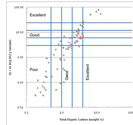
Figure 9. A kerogen quality diagram (Dembicki, 2009) constructed from the Total Organic Carbon (TOC) versus the mass of existing (S1) and potential (S2) hydrocarbons contained in samples of the Tyler Formation. The samples are from the Government Taylor A-1 (green circles) and the State of North Dakota #41-36 (red squares).
