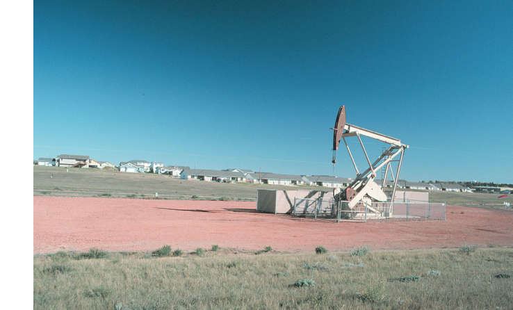
A "horse head" pump lifts oil from the Lodgepole Formation in the southwestern portion of the city of Dickinson.
