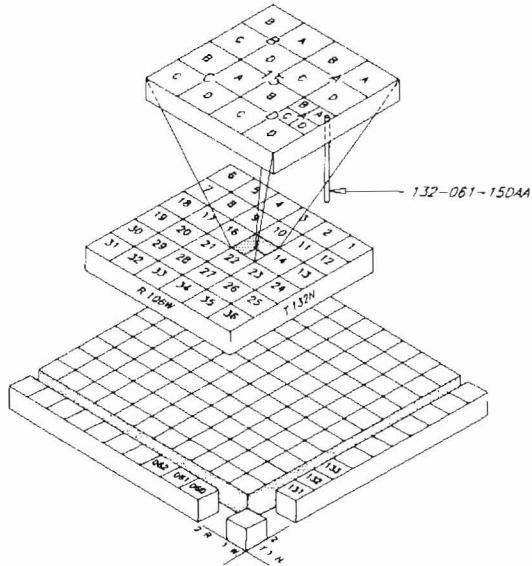
**Figure 9.** The system used to locate wells, test holes, and outcrop locations in this report.
