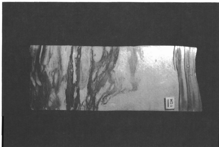
Figure 28. Core slab of a laminated and bioturbated quartzarenite. 5031.3 to 5030.5 feet.
