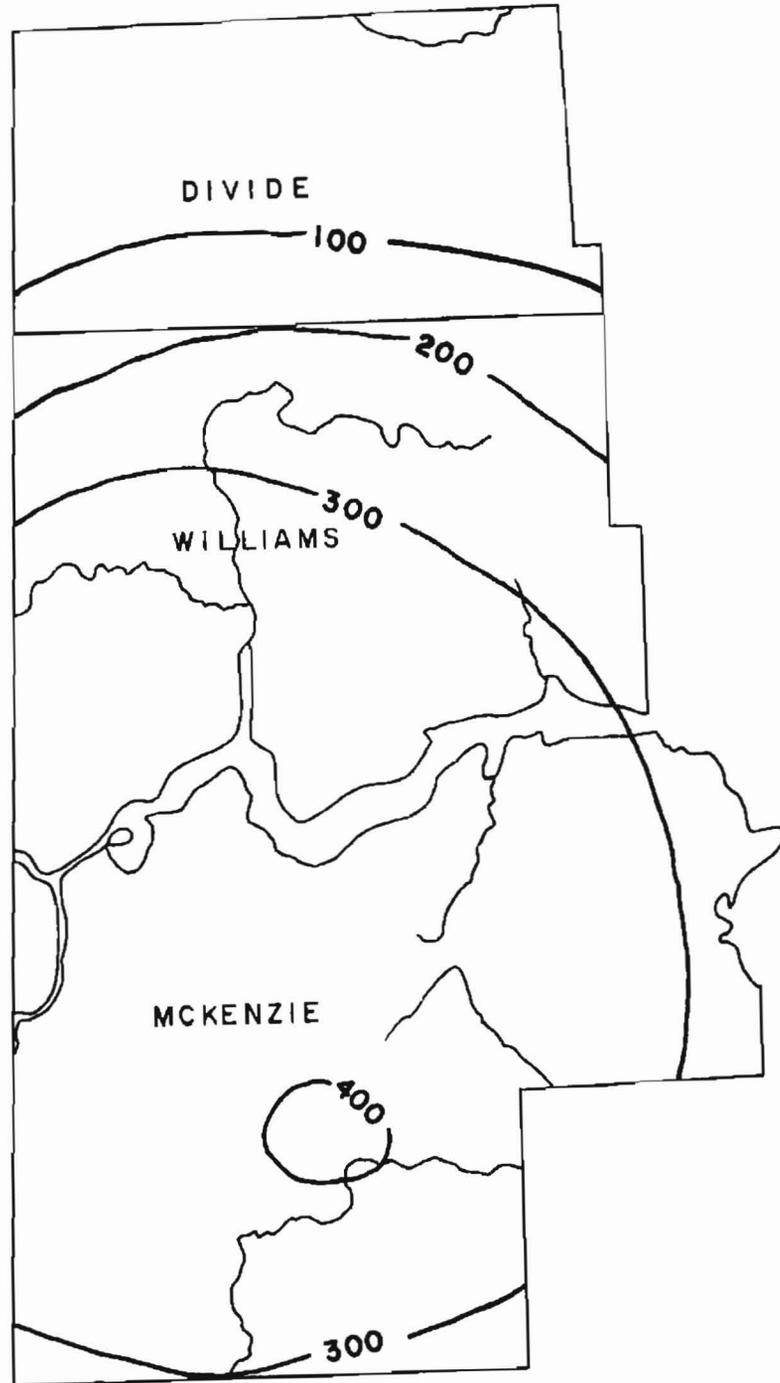
Figure 3. Aggregate thickness in feet of six salt beds in the Charles Formation.
