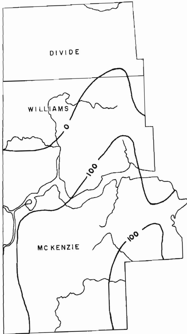
Figure 5. Thickness in feet of the Pine Salt in the Spearfish Formation.
