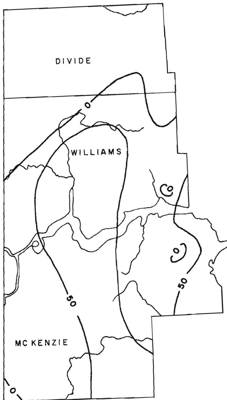
Figure 6. Thickness in feet of the Triassic Dunham Salt.
