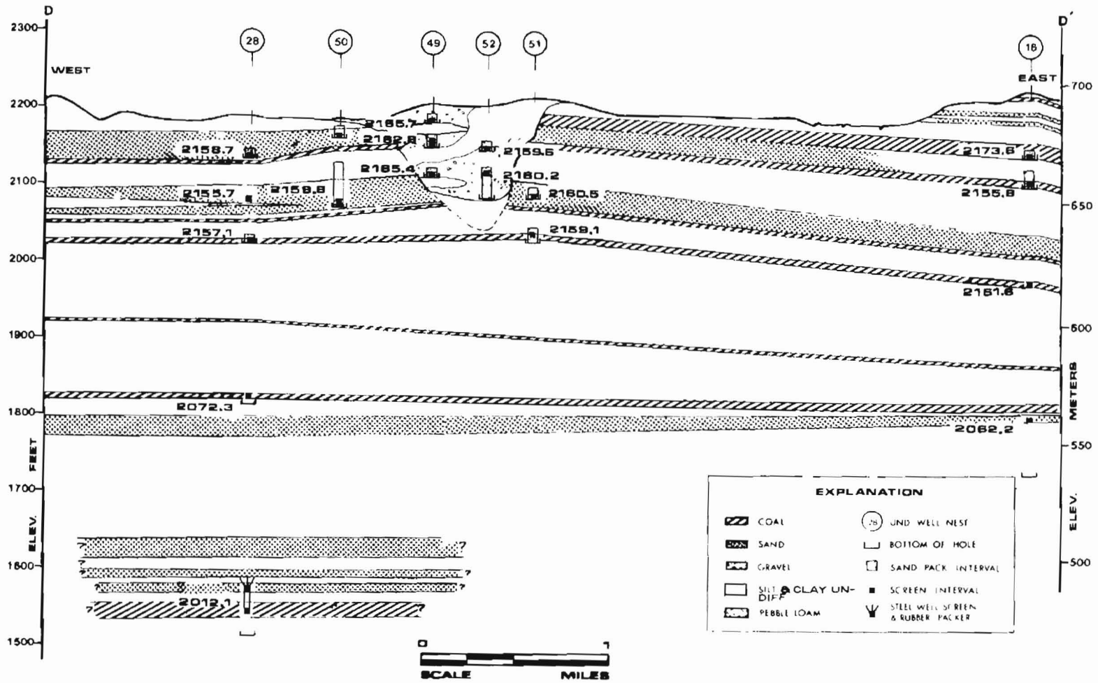
Figure 3.6.4-11 Hydraulic head distribution from observation wells along cross section D-D'. Hydraulic conductivity values times 10^{-4} cm/sec. Location of the cross section shown on figure 2.1.10-2.
