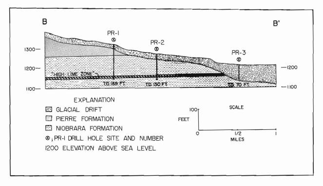
Figure 5 - Cross-section along the line B - B' showing geology of the Park River prospective area.
