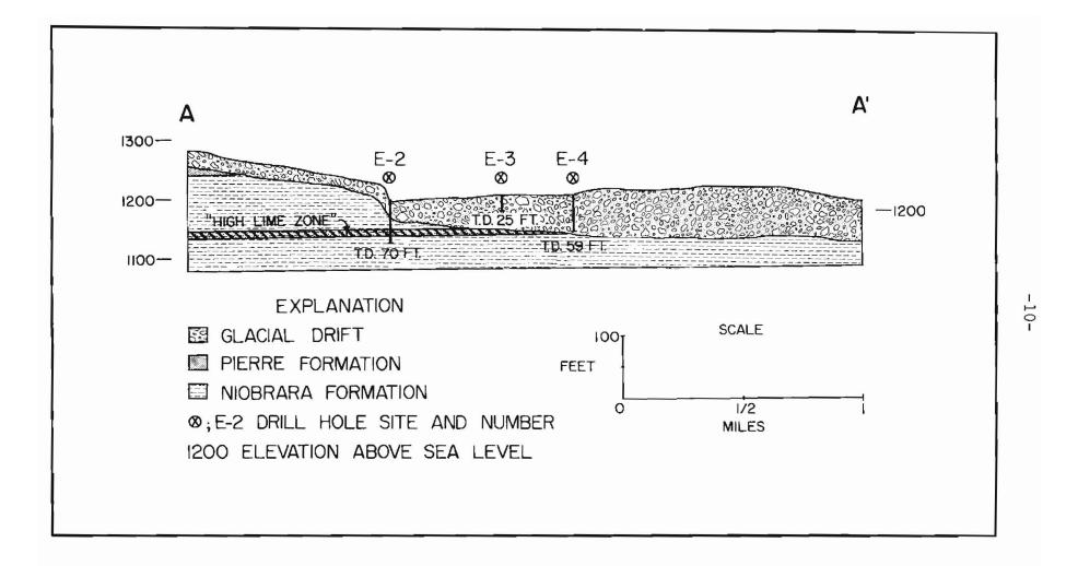
Figure 3 - Cross-section along the line A - A' showing geology of the Edinburg prospective area.
