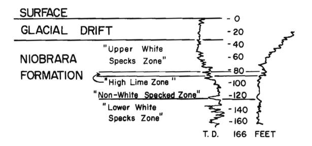
Test Hole PR-1; Location - NE NE Sec. 25, T. 157 N., R. 57 W., Walsh County, North Dakota. Elevation - 1313. Total Depth - 169 feet.
