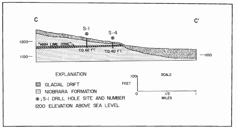
Figure 9 - Cross-section along the line C - C' showing geology of the Shawnee-McCanna prospective area.
