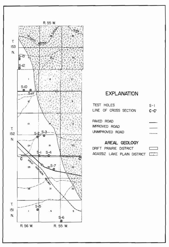
Figure 6 - Map of the Shawnee-McCanna prospective area showing test hole locations, general geology of the area and the line of cross-section.
