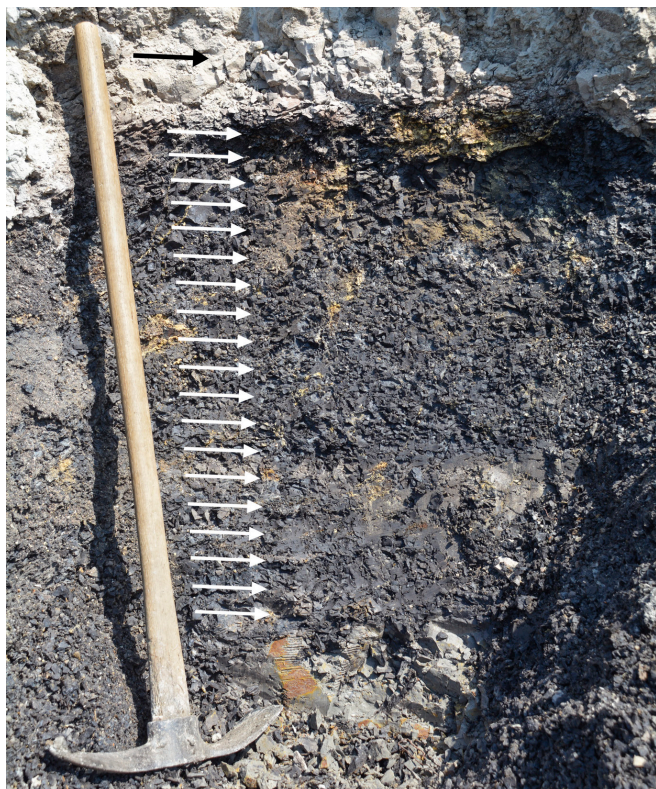
Figure 21. Nineteen inches (46 cm) of black claystone at measured section 123 (T136N, R102W, Sec. 8). Each vertical inch (2.5 cm) was collected in 2 kg (4.4 lb.) samples (white arrows) until the claystone became medium gray. One sample of the overlying light gray mudstone roof (Rhame bed weathering zone) was also collected (black arrow).
