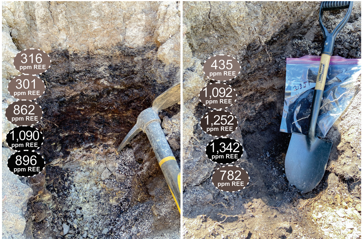
Figure 24. Sampling at measured sections 210 (left) and 213 (right), 400 feet (120 m) apart in T136N, R102W, Sec. 22. The carbonaceous material was 15 inches (38 cm) thick at section 210 and 22 inches (56 cm) thick at section 213. Five samples were taken vertically through the bed at each location. Results show that the lignite within the Rhame bed weathering zone in this area contains higher REE concentrations near the bottom than at the top of the bed, which is unusual compared to other sampling locations. This is likely because the highest-grade lignite occurs closer to the bottom of the bed at these sites, and the top is uncharacteristically more clay-rich.
