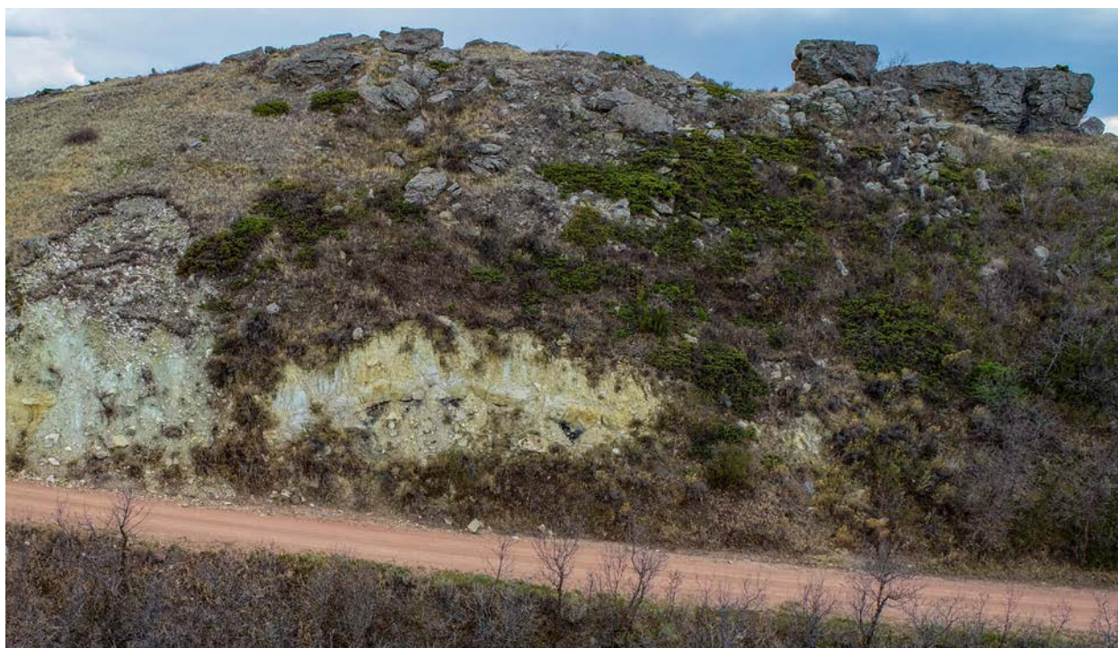
▲ Figure 14. Measured section 28 at Sentinel Butte. Samples were taken from the uraniumiferous coal exposed below the yellow sandstone exposed in the center of the photo. Drone photo taken looking southwest.
