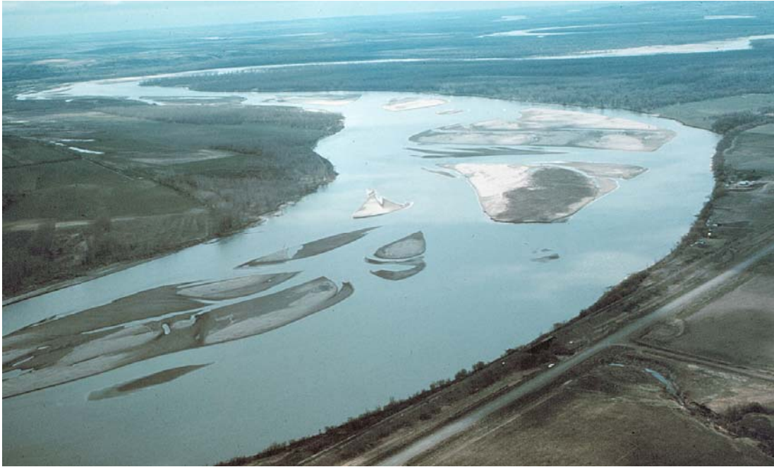
Figure 19. View to the southeast of sand bar deposits in the Missouri River channel at south Bismarck. Seasonal variations in flow help to modify the location and extent of these types of deposits.
