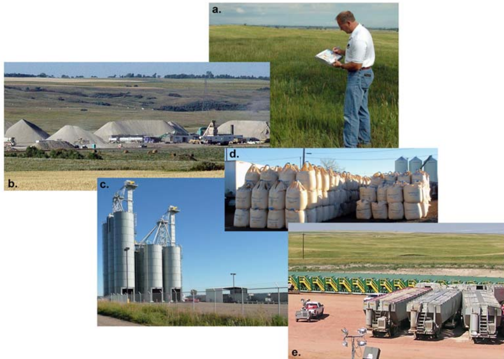
Figure 4. Illustration of several of the steps in the production of a sand resource for use as a proppant: a. identification and mapping of potential sand resources in the field, b. contemporary sand and gravel processing operation, c. bulk transfer facility from rail delivery to truck transport, d. staging proppants in distribution areas for transport to the well site, e. rail cars of proppant sand and frac tanks staged on the well pad.
