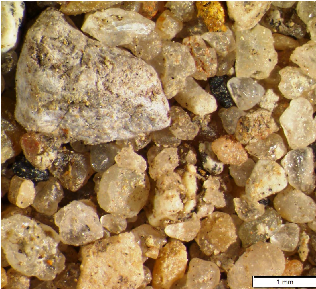
Figure 10. Bulk sample photomicrograph (25x) of glaciofluvial sand from the Verendrye glaciofluvial meltwater diversion channel southeast of Velva, North Dakota.
