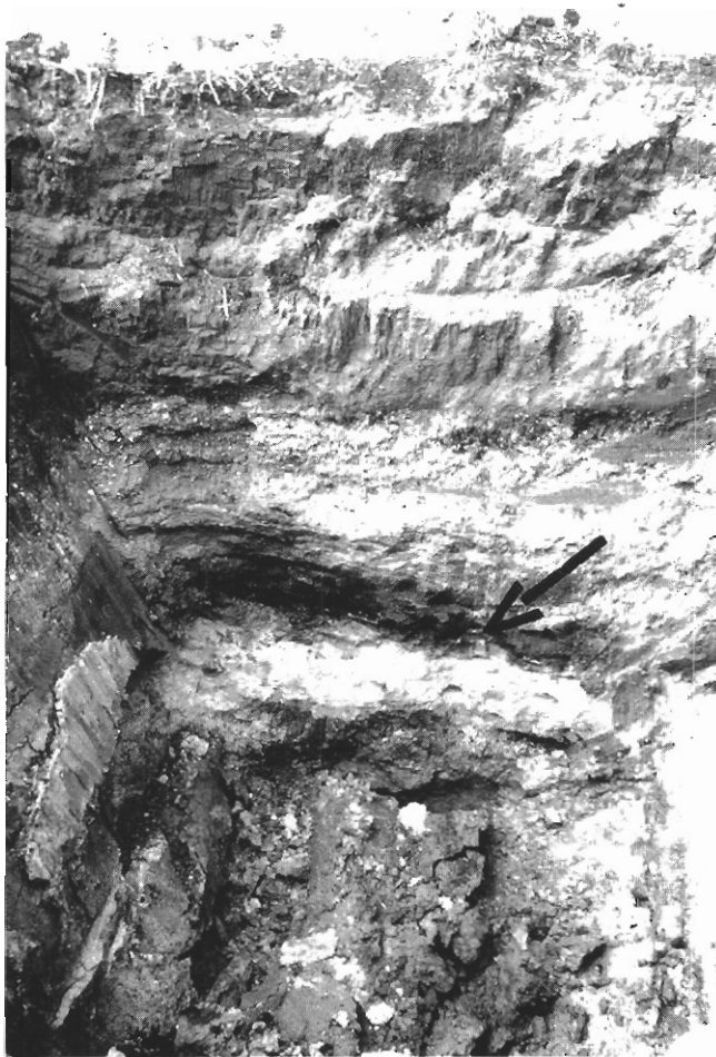
Figure 10. Sediment exposed on the west wall of trench JT1 in the Jerusalem Outlet. Arrow points to a paleosol. The trench was 9 feet deep at the time this photo was taken.
