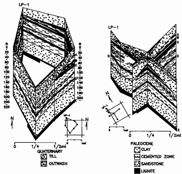
Figure 6. Fence diagram and a monitoring well nest at the Black Slough Field, Burke County, North Dakota.
