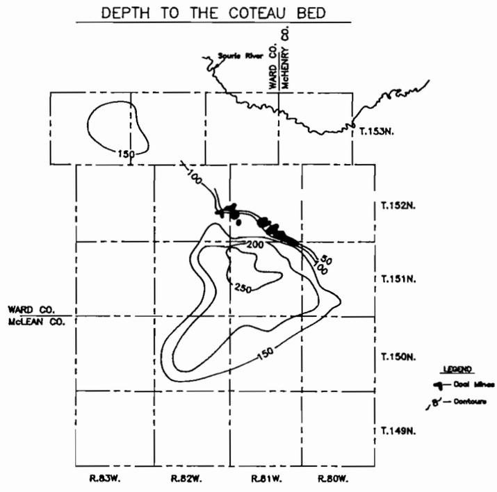
Figure 10. Isopach and overburden thickness map of the Coteau bed in Ward and McHenry counties.
