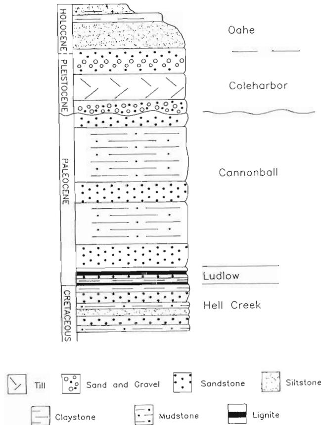
Figure 2. Generalized stratigraphic column for sediments and sedimentary rock exposed at the surface in the Bismarck-Mandan area.
