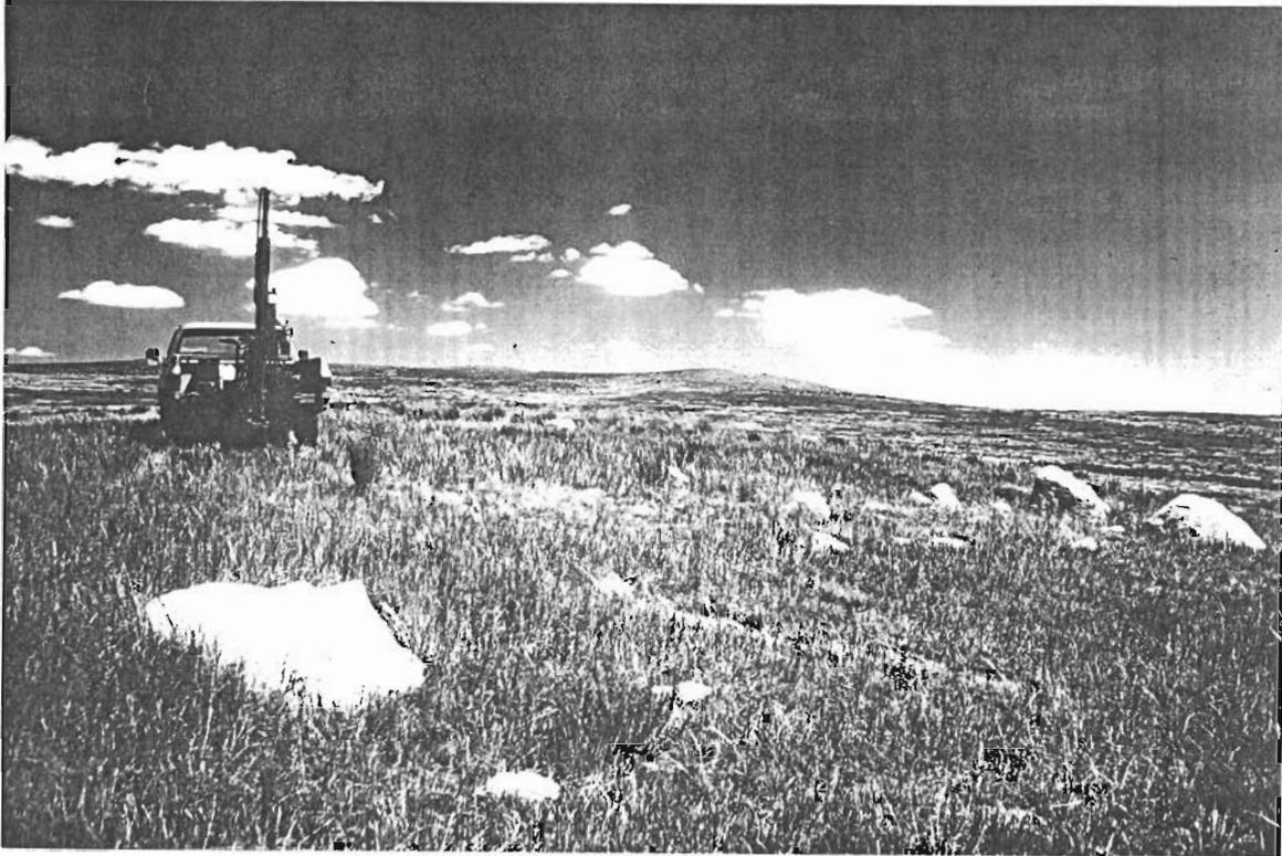
*Figure 3. Truck-mounted Giddings soil probe used during this project. The truck is pictured north of Bismarck (T139N, R80W, section 18 nwswe).*
