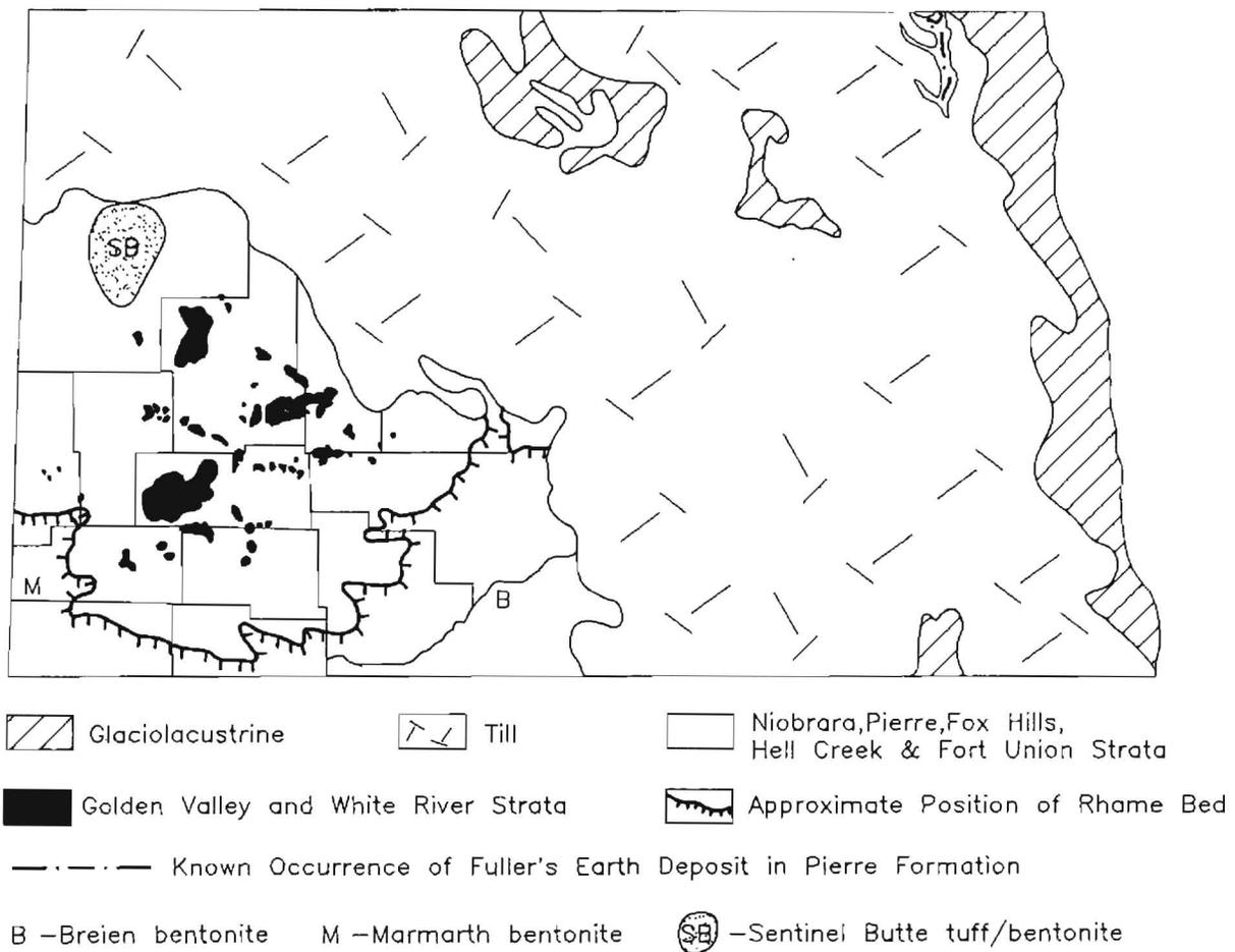
**Figure 2.** A generalized geologic map of North Dakota (modified from Bluemle, 1977 and Clayton, 1980).
