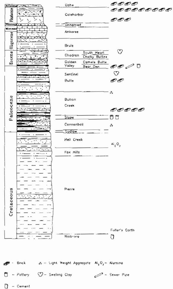
**Figure 1.** The upper portion of the generalized stratigraphic column of North Dakota. The symbols indicate the general stratigraphic position of clay and claystone utilization in North Dakota.
