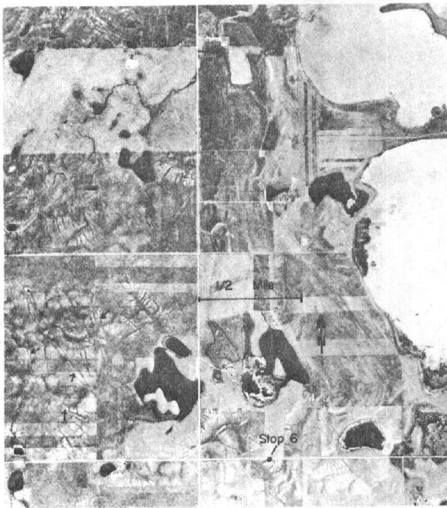
Figure R-16. Air photo of typical collapsed superglacial alluvium with disintegration trenches (arrows) around stop 6 on fig. R-17. (U.S. Dept. of Agriculture BAD-2K-19 7-3-52.)
