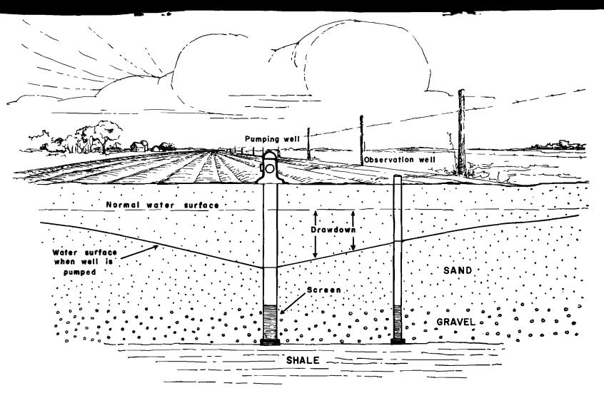
FIGURE 6. SUBSURFACE CONDITIONS IN VICINITY OF PUMPING WELL
