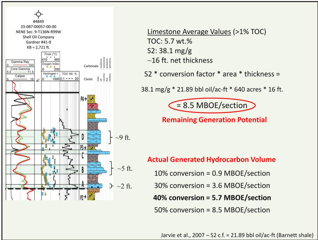
Approximately 5.7 million barrels of oil per 640 acres may have been generated from the organic-rich, upper Tyler limestone beds within the area of the Gardner #41-9 (assuming 40% kerogen conversion based on thermal modeling and Tmax values).
