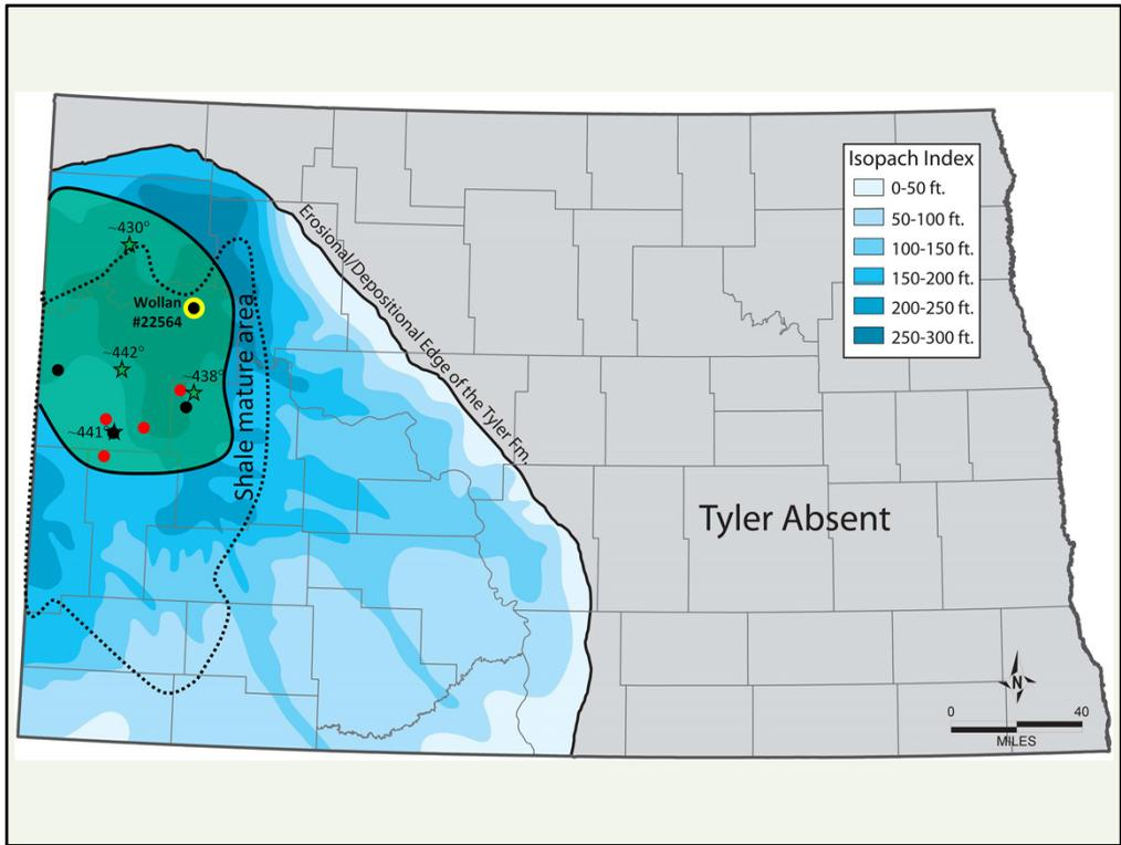
All of the successful DST's and productive vertical wells to date are located within the Tyler's modeled area of thermal maturity. There is currently no evidence of significant hydrocarbon migration within or out of the northern Tyler petroleum system. Perhaps the peripheral to southern areal extents of the northern Tyler source beds are more favorable to conventional, and possibly unconventional, exploration.
