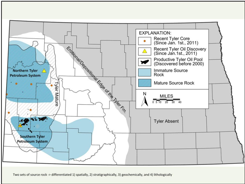
The Tyler Formation contains two separate petroleum systems where two sets of unique source rock can be differentiated spatially, stratigraphically, geochemically, and lithologically. These two source rock sets and their respective stratigraphic sequences are the focus of this presentation.
