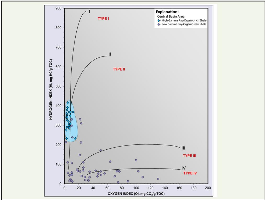
Hydrogen and oxygen index values measured from core samples of the high gamma ray shale beds plot along a Type I/II kerogen curve on a modified Van Krevelen diagram, indicating these source beds are prone to generating oil.
