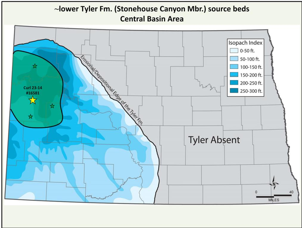
The Tyler core from Whiting's Curl 23-14 (yellow star) is currently the longest, most complete core of the Tyler Formation in the central, deeper portions of the Williston Basin (the green shaded area represents the approximate extent of the primary source beds in the Tyler's northern petroleum system).
