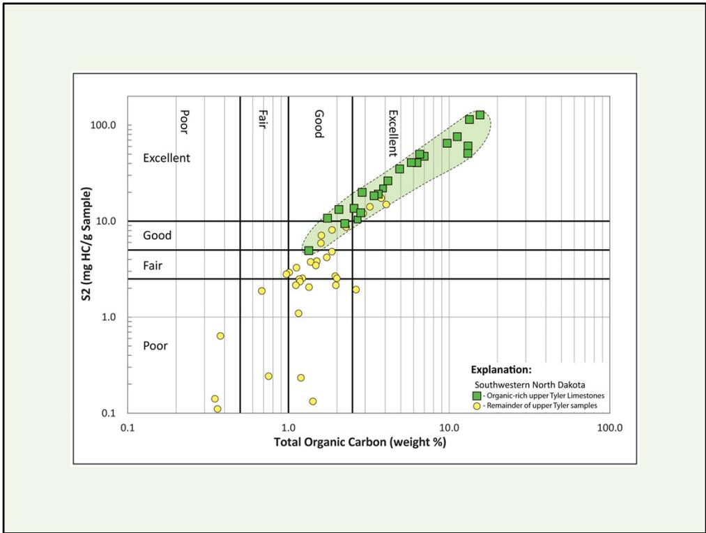
On an organic-richness plot, the organic-rich limestone bed samples plot as good to excellent quality source rock along with some of the interbedded shale samples.
