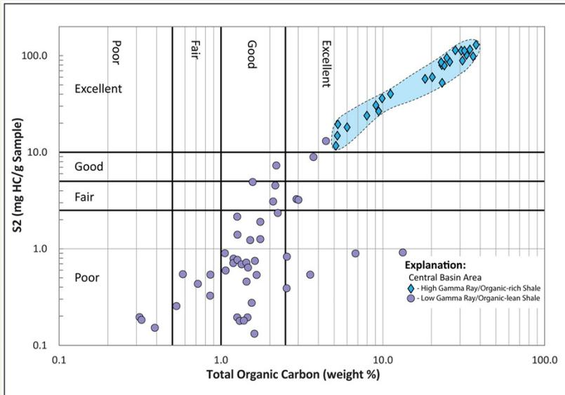
Most core samples from the high gamma ray shale beds plot as excellent quality source rock, both in terms of TOC wt. % and S<sub>2</sub> content. Samples from the remaining low gamma ray shale sometimes plots as fair to good quality source rock, but due to low S<sub>2</sub> values generally classify as poor quality source rock.
