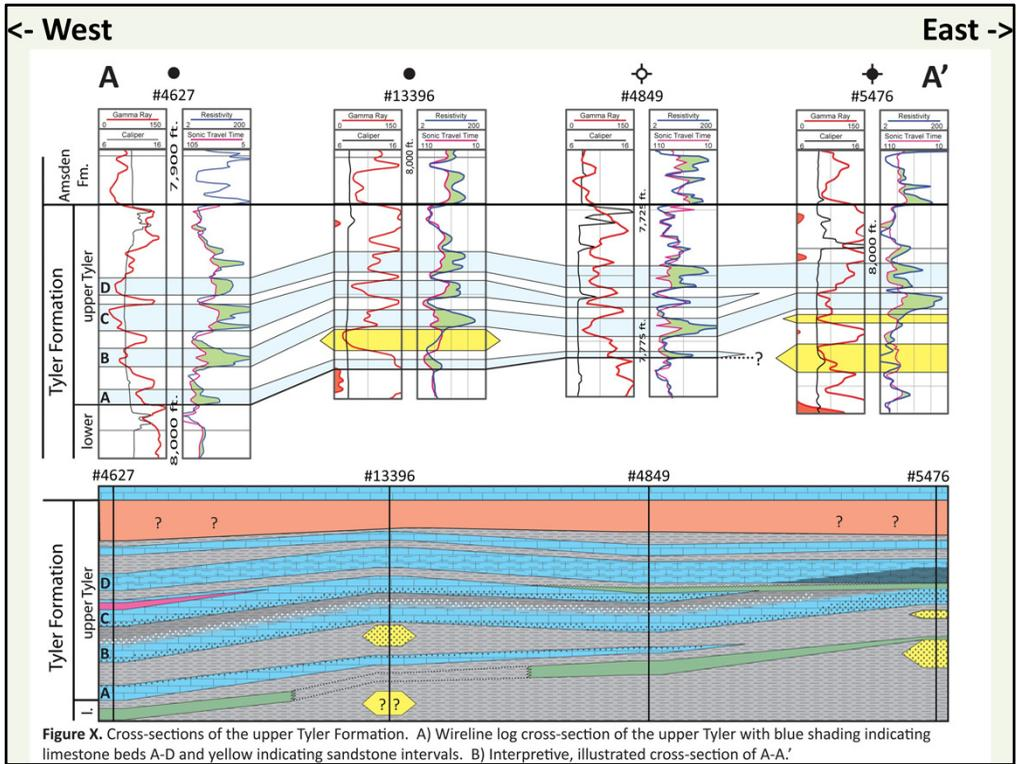
Figure X. Cross-sections of the upper Tyler Formation. A) Wireline log cross-section of the upper Tyler with blue shading indicating limestone beds A-D and yellow indicating sandstone intervals. B) Interpretive, illustrated cross-section of A-A'.
