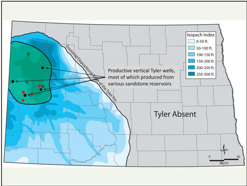
Four productive vertical Tyler wells from this northern area (black dots) are all located along the peripheral extent of the high gamma ray, very organic-rich shale intervals.
