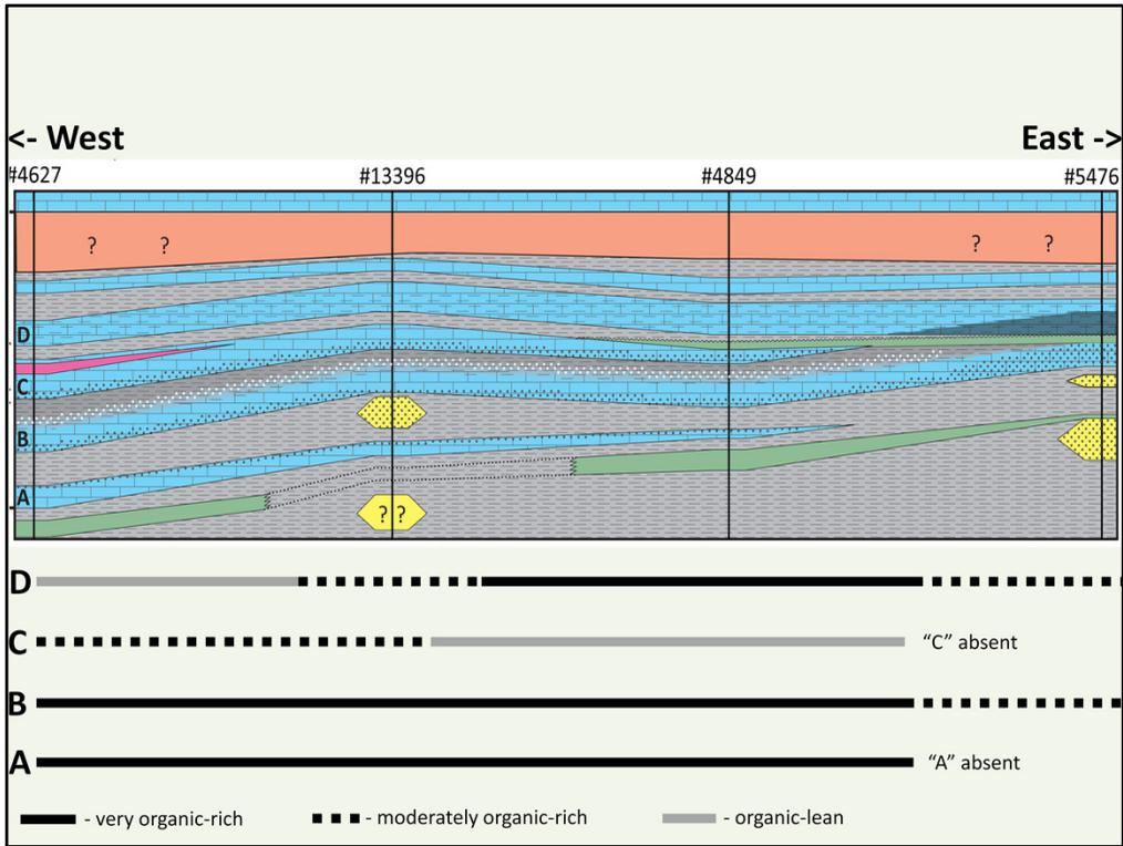
Based on core observations, geochemical core data, and wireline log signatures (sonic log), there appear to be areas where at least three of the limestone beds are organic-rich. In other areas, these limestone beds are absent and/or transition to moderate to poor quality source beds.
