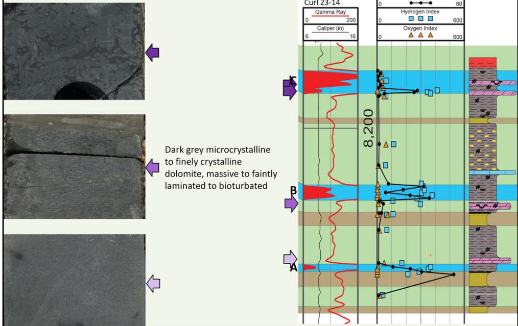
Thin, dark grey, microcrystalline dolomite layers are also present which are all located in close stratigraphic proximity to the high gamma ray shale intervals. These finely crystalline dolomites vary in texture from being faintly laminated to massive to bioturbated.
