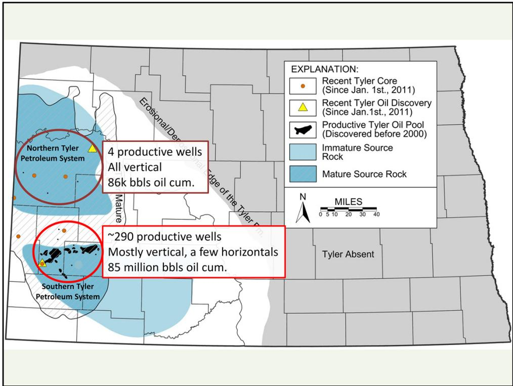
The northern petroleum system appears to lack significant quantities of conventional reservoir, which is why there have only been four productive wells in the system to date. The southern petroleum system contains oil productive bar-type and channel sandstone reservoirs that have been successfully explored and developed over the past 50+ years.
