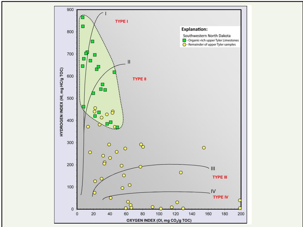
On a modified Van Krevelen diagram, samples from the organic-rich limestone beds plot along a Type I/II kerogen curve indicating they are prone to generating oil. Most of these samples yielded Tmax values of 440-445° indicating they are thermally mature and have undergone intense oil generation. Some of the interbedded shale intervals (yellow circles) also plot along a Type I/II kerogen curve.
