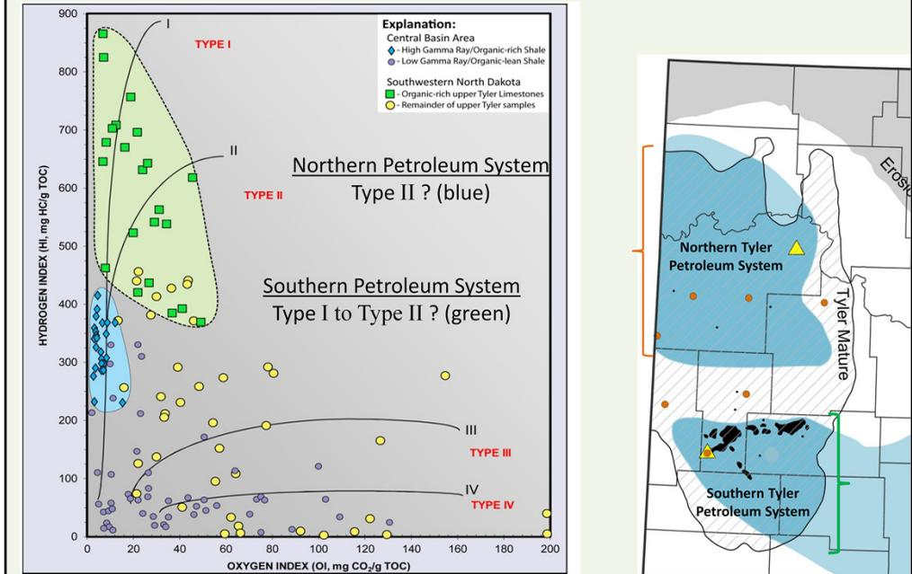
While samples from both sets of source beds plot along a Type I/II kerogen curve, they differentiate into two separate populations which suggests different types of organic-matter. Different types of organic matter would explain the differences in oils produced from the two systems (the paraffin concentrations varies from 20-40% in the southern system to <5% in the northern system) and also could mean differences in maturation parameters.
