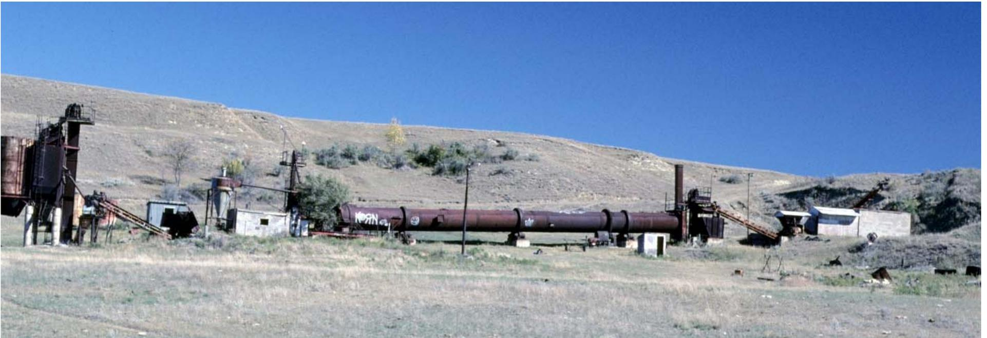
One of the Griffin rotary kilns was moved to Lehigh in Stark County to make clay aggregate. Today, this equipment still contains elevated levels of radioactivity.
