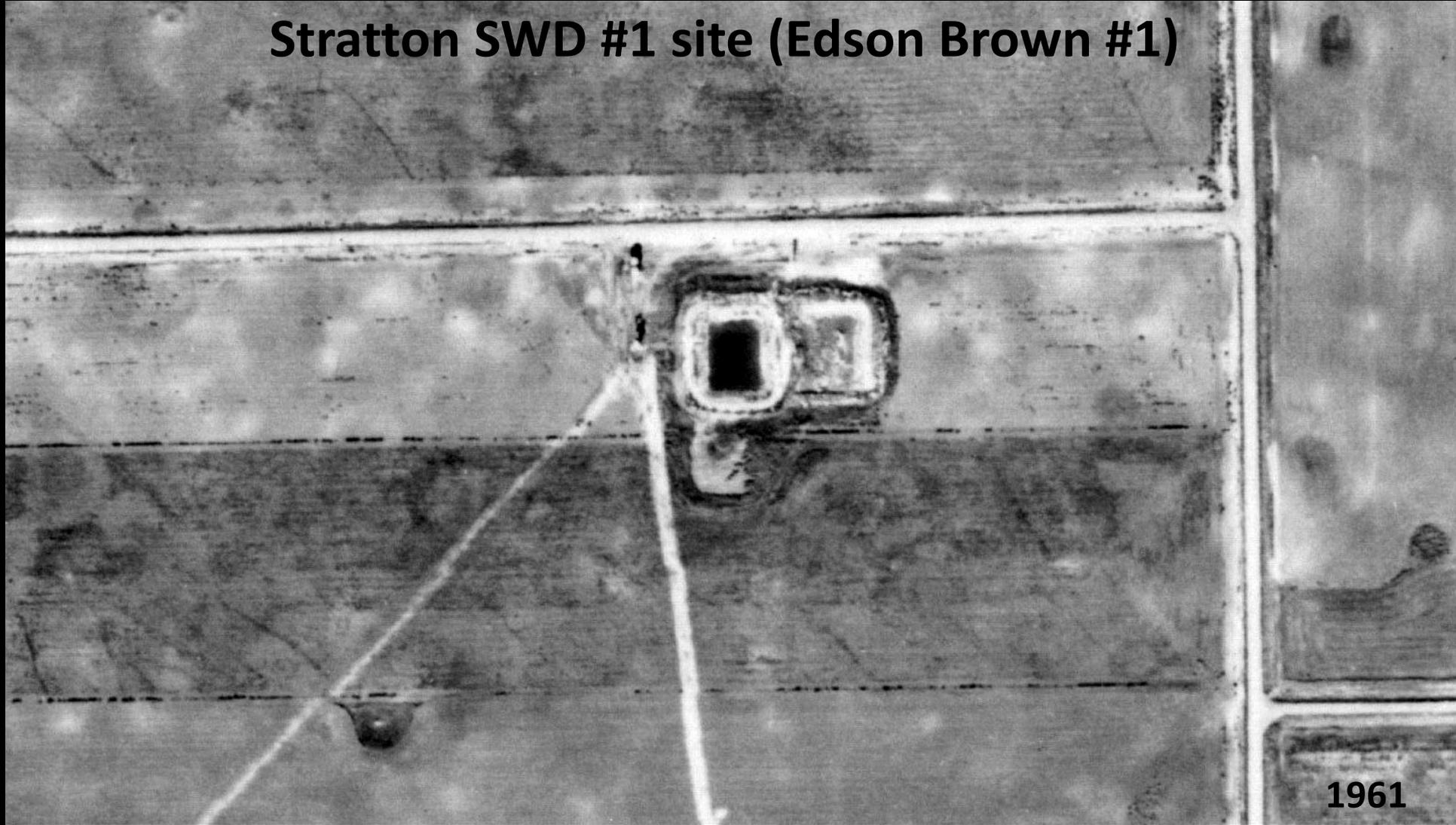
The site contained two brine holding ponds from 1959 to at least 1970 (with dimensions of 100 x 90 ft and 60 x 100 ft and 5 feet deep). Produced 178,000 barrels of saltwater.
