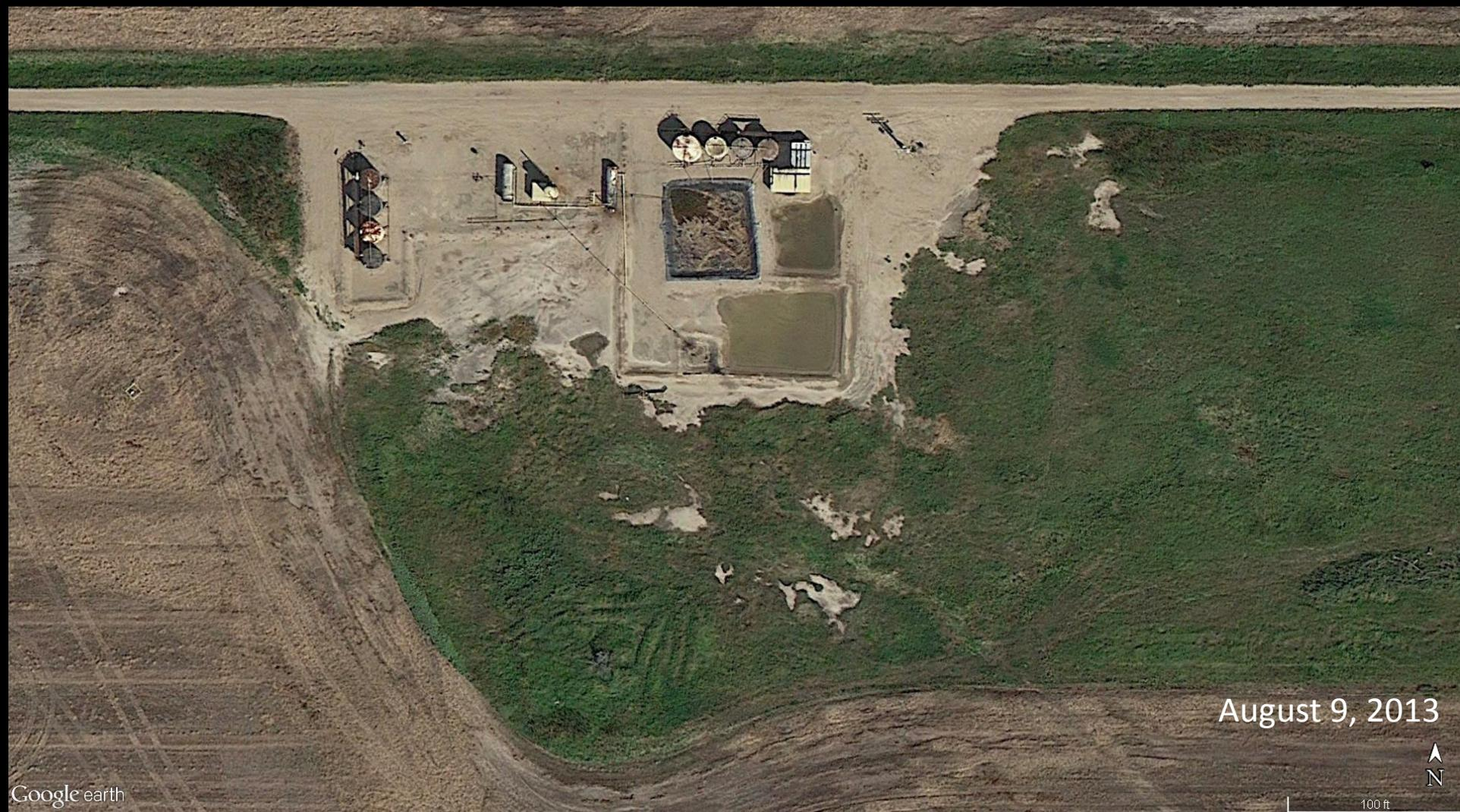
Drilled in 1959 by Cardinal Petroleum (Edson Brown #1). Produced oil from 1959-1970. Converted to a saltwater disposal well by Phillips Petroleum in 1978 (Stratton SWD #1).
