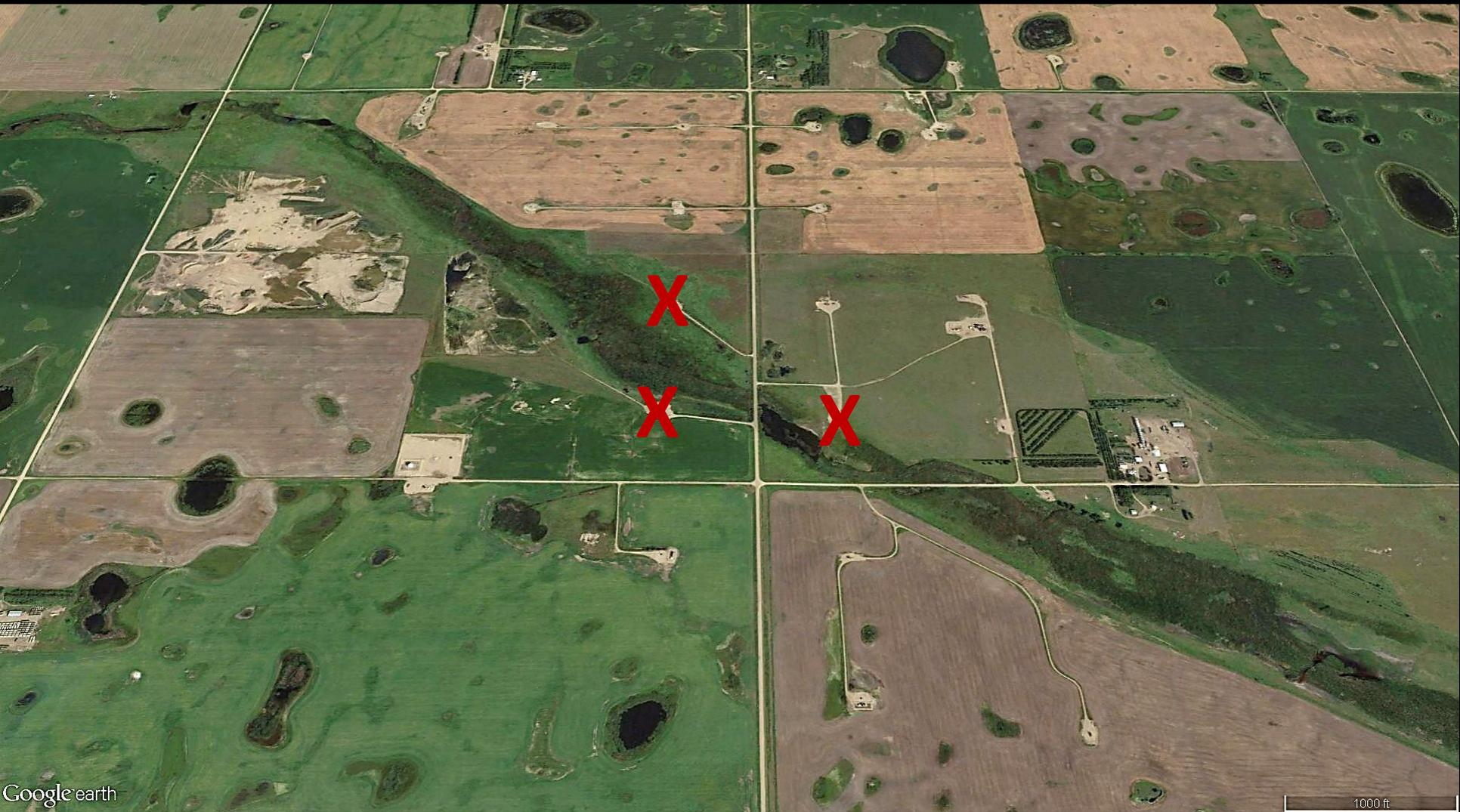
Under today's rules, these locations (X) would require a closed mud system due to a **high watertable** and **near surface sand and gravel** deposits.
