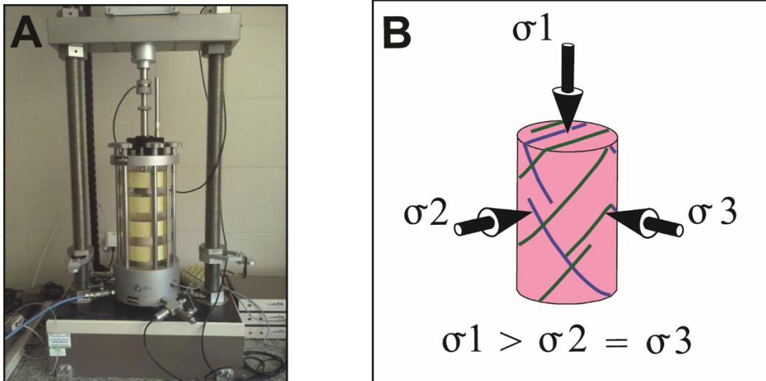
**Figure 1.** (A) Apparatus used for triaxial compression rock deformation experiments. (B) Schematic of stress states for triaxial deformation.  $\sigma$ -sigma.
