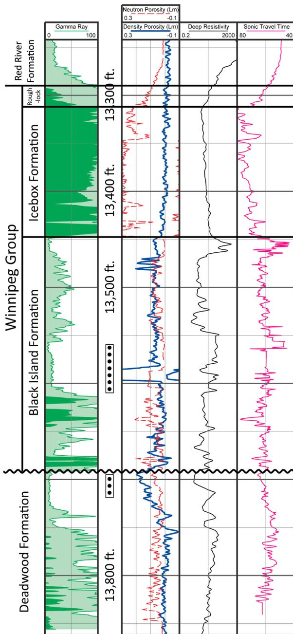
**Figure 10.** Wireline logs with perforation and production information for Amerada Hess’s Pederson #14-22. Note: the Pederson #14-22 was renamed the Astrid Ongstad 14-22. The Pederson #14-22 well location is depicted as a yellow star on the Figure 6 map.
