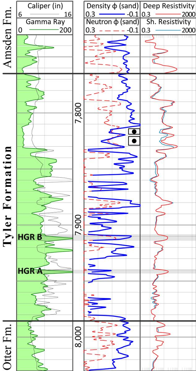
Figure 9. Wireline logs of the Tyler Formation section from Pennzoil's Federal #18-44 showing the perforated intervals (outlined black dots).
