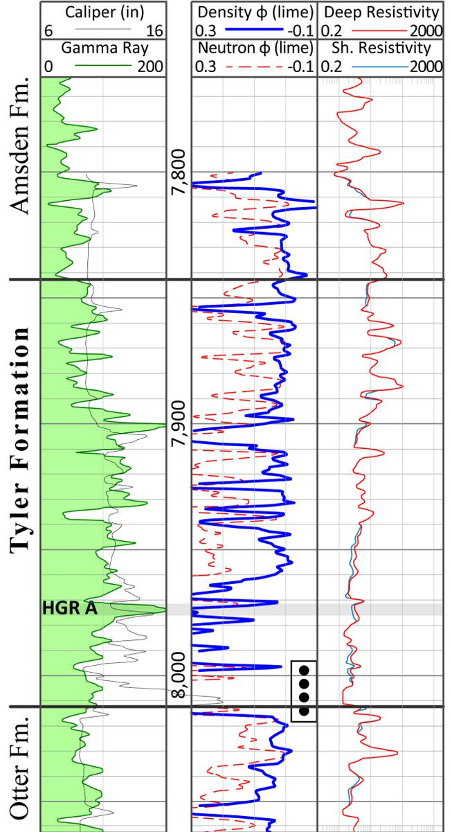
Figure 10. Wireline logs of the Tyler Formation from Supron Energy's F-7-144-101 #1 showing the perforated interval (outlined black dots).
