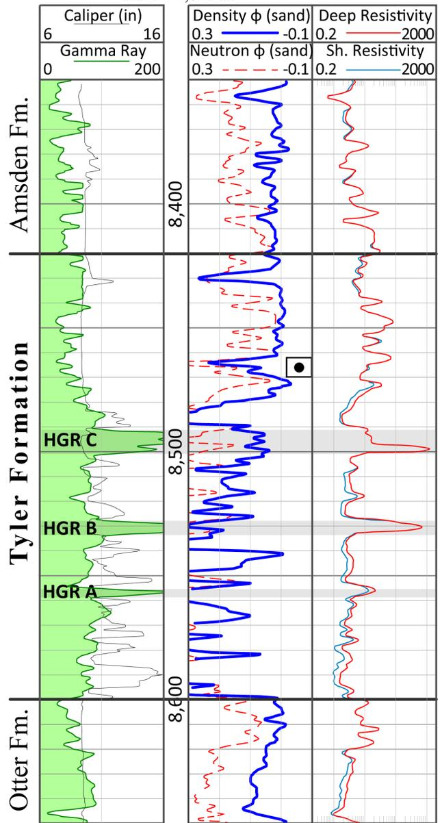
Figure 12. Wireline logs of the Tyler Formation from Pennzoil's Grassy Butte #16-33 showing the perforated interval (outlined black dot).
