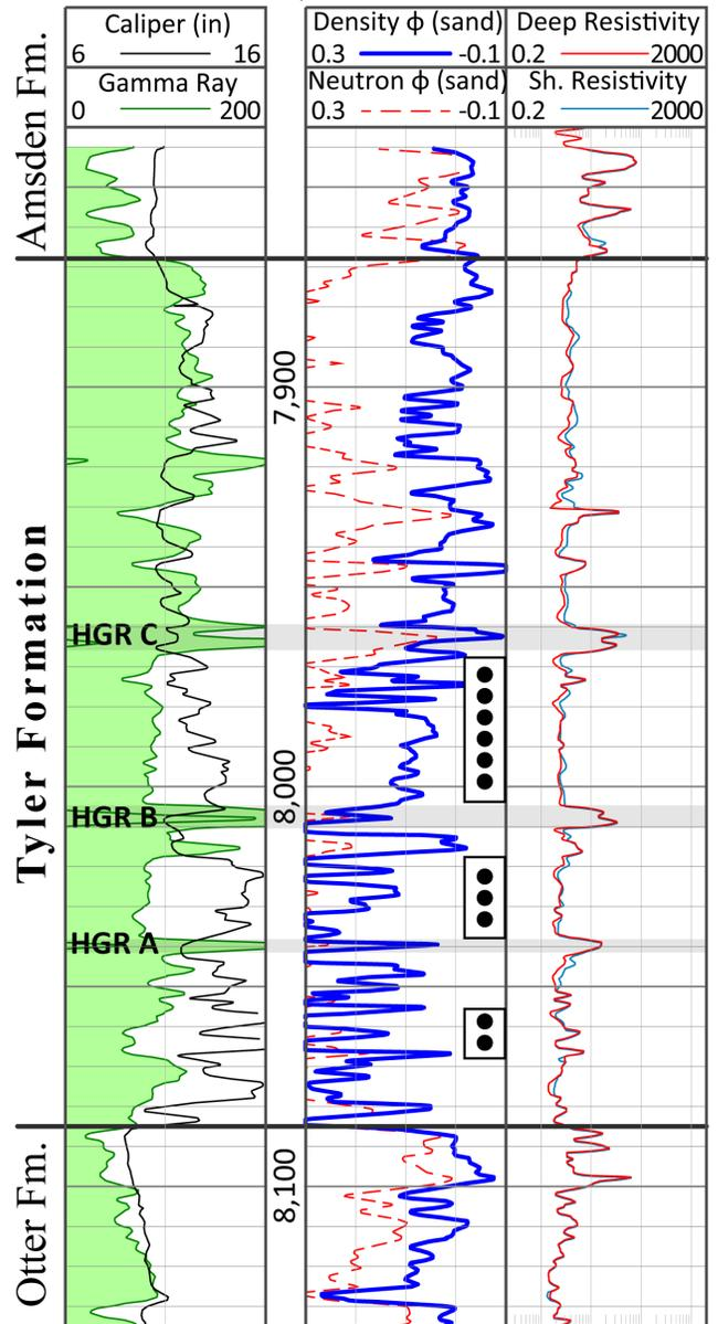
Figure 14. Wireline logs of the Tyler Formation from UMC Petroleum's Jeffrey #33-33 showing the perforated intervals (outlined black dots).
