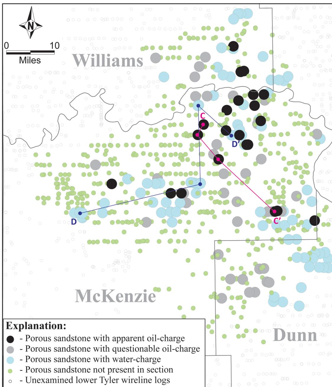
**Figure 16.** Map of the study area showing the distribution of wells with wireline logs that were examined for porous sandstones.
