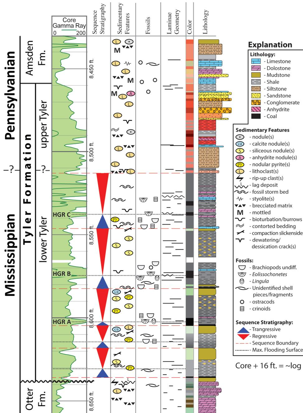
**Figure 4.** Example core illustrated (right) with core gamma-ray (left) of the Tyler Formation from Continental Resources Morison 1-14H (NDIC #22104, API: 33-053-03913-00-00, Sec. 14-T148N-R99W) located in central McKenzie County.
