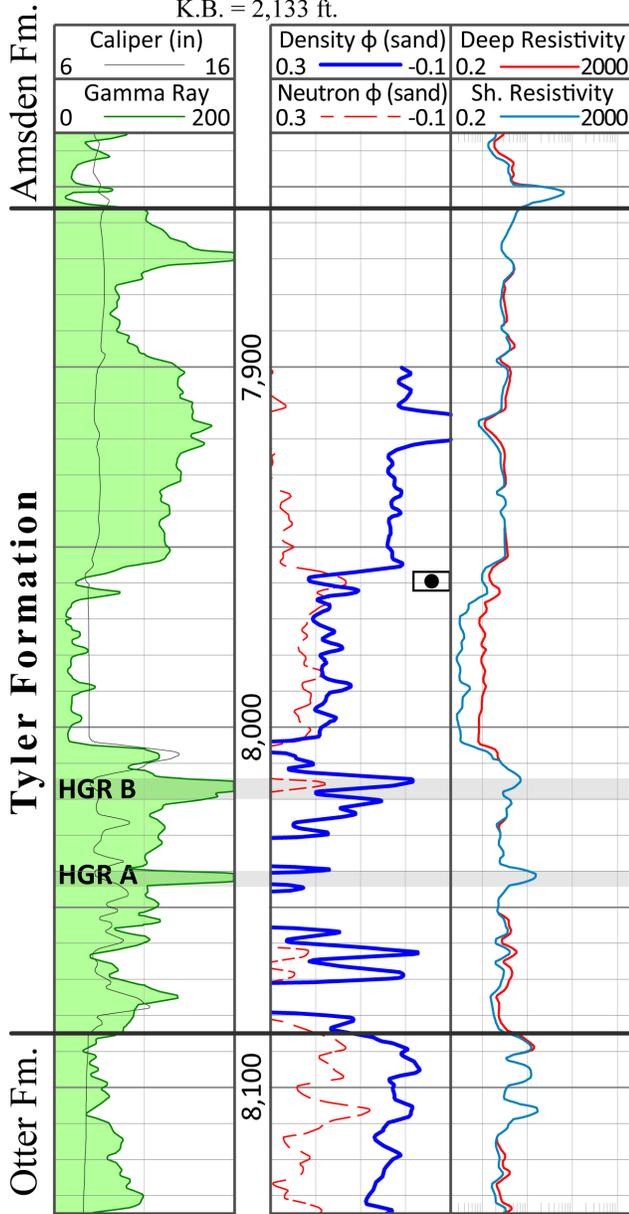
Figure 13. Wireline logs of the Tyler Formation from Columbus Energy's Bertinuson #1-31 showing the perforated interval (outlined black dot).
