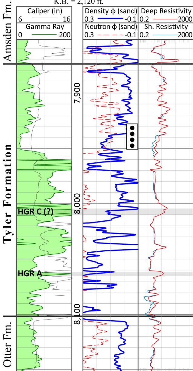
Figure 11. Wireline logs of the Tyler Formation from Gulf Oil's Carus #3-30-2B showing the perforated interval (outlined black dots).
