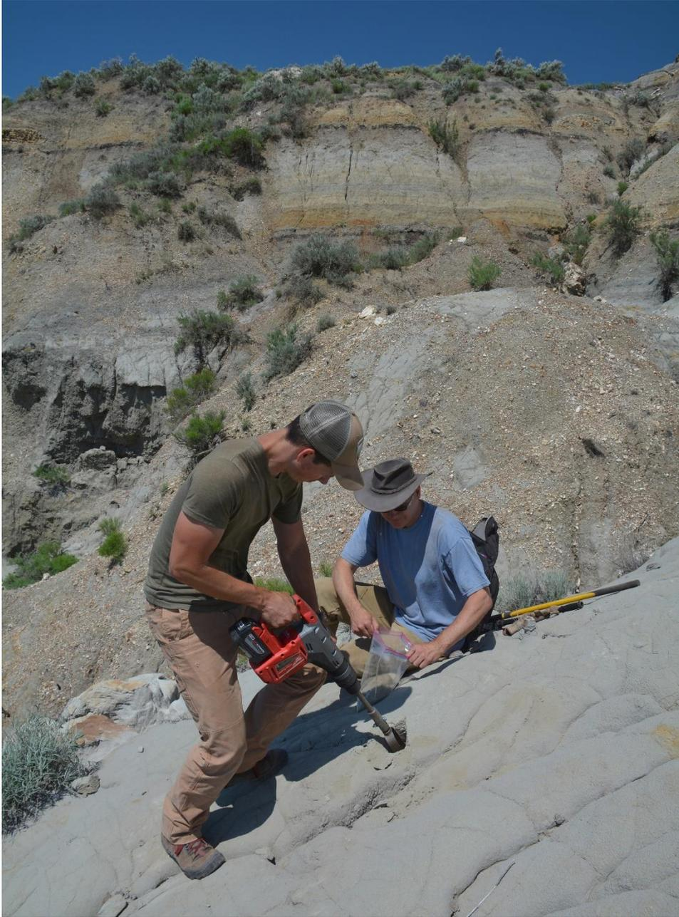
**Figure 3.** Bedrock sandstone sample collection on an outcrop of Sentinel Butte Formation using a battery-operated hammer drill. Using this portable coring device permits sampling below the weathered zone of the outcrop, providing a better representative sample of the sandstone for testing and characterization. The custom fabricated three-inch diameter coring barrel permits rapid collection in semi-cemented rocks.
