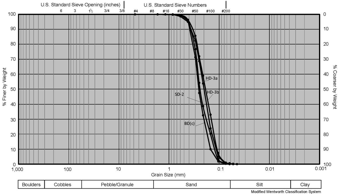
**Figure 11.** Gradational curves of sand from the Hazen-Stanton Dunes. Steep curves like this are indicative of samples that are well sorted and contain a relatively small range of grain sizes.
