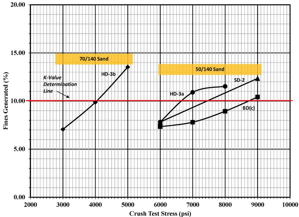
**Figure 10.** Crush resistance curves for eolian sands tested from the Hazen, Stanton, and Basto Dunes. K-Value determinations are found at the point where 10% or more of fines are generated upon crush rounded down to the nearest 1000 psi.
