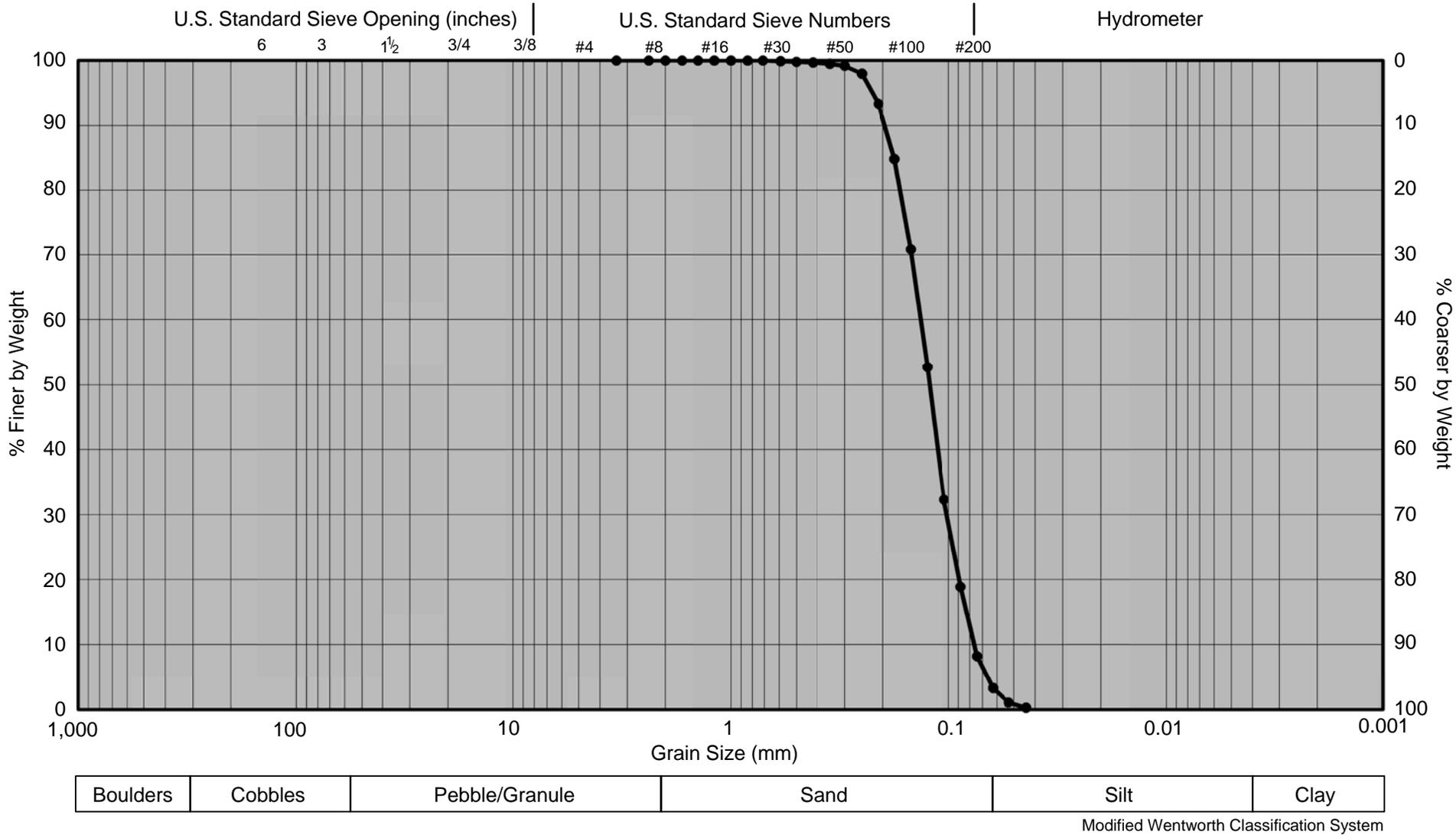
Figure 34. Bulk Sample Grain-Size Distribution Diagram for Sample No. 1 - Qod.
