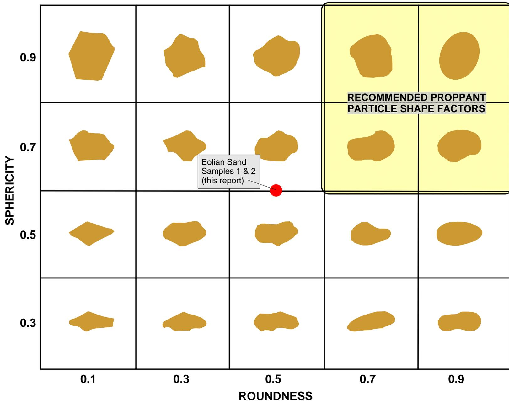
Figure 39. Sphericity and roundness chart displaying the range of recommended proppant particle shape factors and values for selected eolian sand samples tested from sand deposits in North Dakota.
