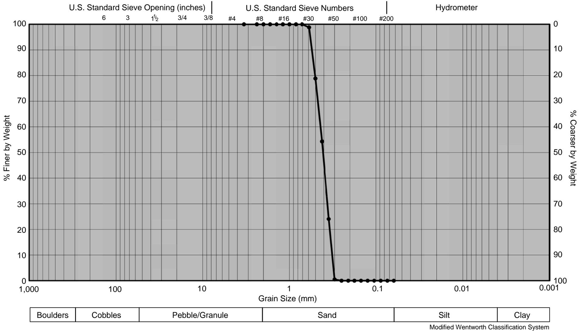
Figure 37. Grain size distribution diagram for Sample No. 2 - Qtou 30/50 Cut.
