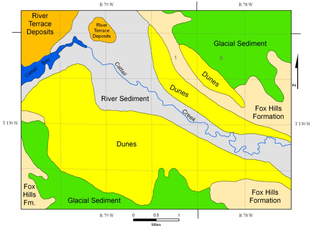
**Figure 9. Map of bedrock and surface geologic units in the southeastern Cattail Bay-Winona Flats area in southwestern Emmons County along the Missouri River. Dunes are present on both the north and south sides of Cattail Creek and resulted when the finer portions of these water-deposited sediments, were reworked by the wind into dunes.**
