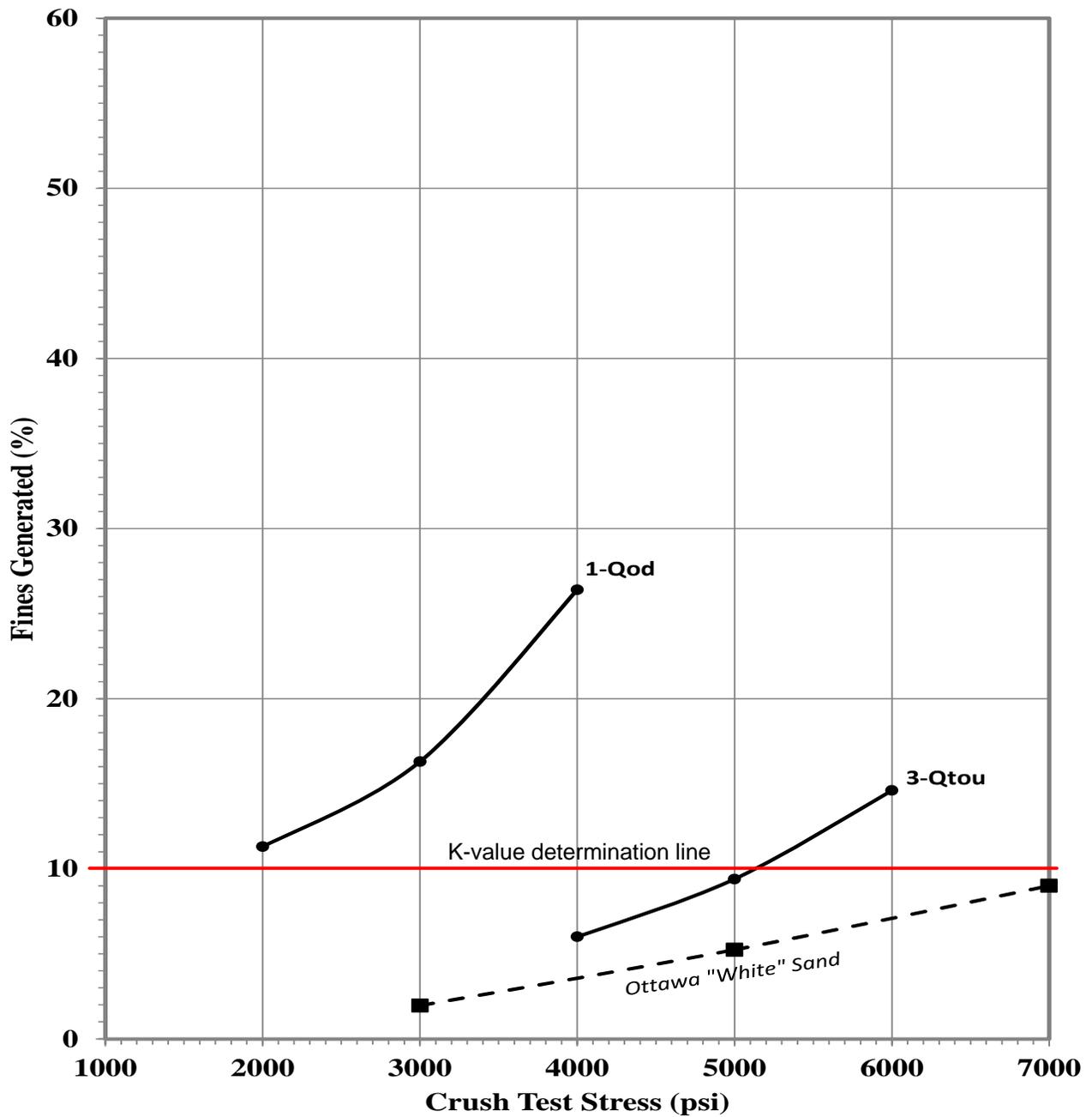
Figure 42. Crush test stress versus fines generated curves for selected eolian sand samples from North Dakota: Sample No. 1 - Windblown Sand (Qod) from the Denbigh Dunes area in McHenry County, Sample No. 2 - Wind-blown Sand (Qtou) of the Denbigh Dunes area in northeastern McHenry County.
