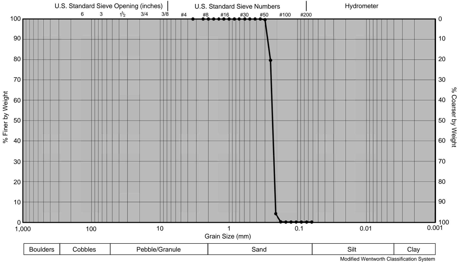
Figure 36. Grain size distribution diagram for Sample No. 1 - Qtou 40/70 Cut.
