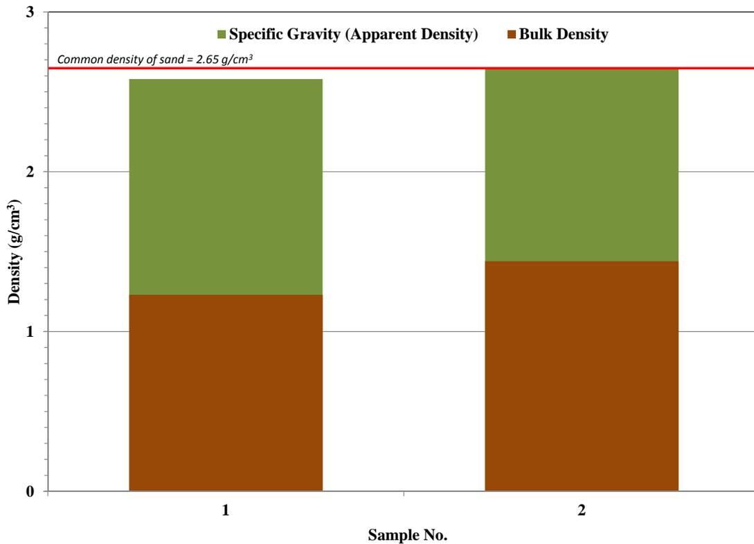
**Figure 44. Comparison of Specific Gravity (apparent density) and Bulk Density values for selected eolian sand deposits.**
