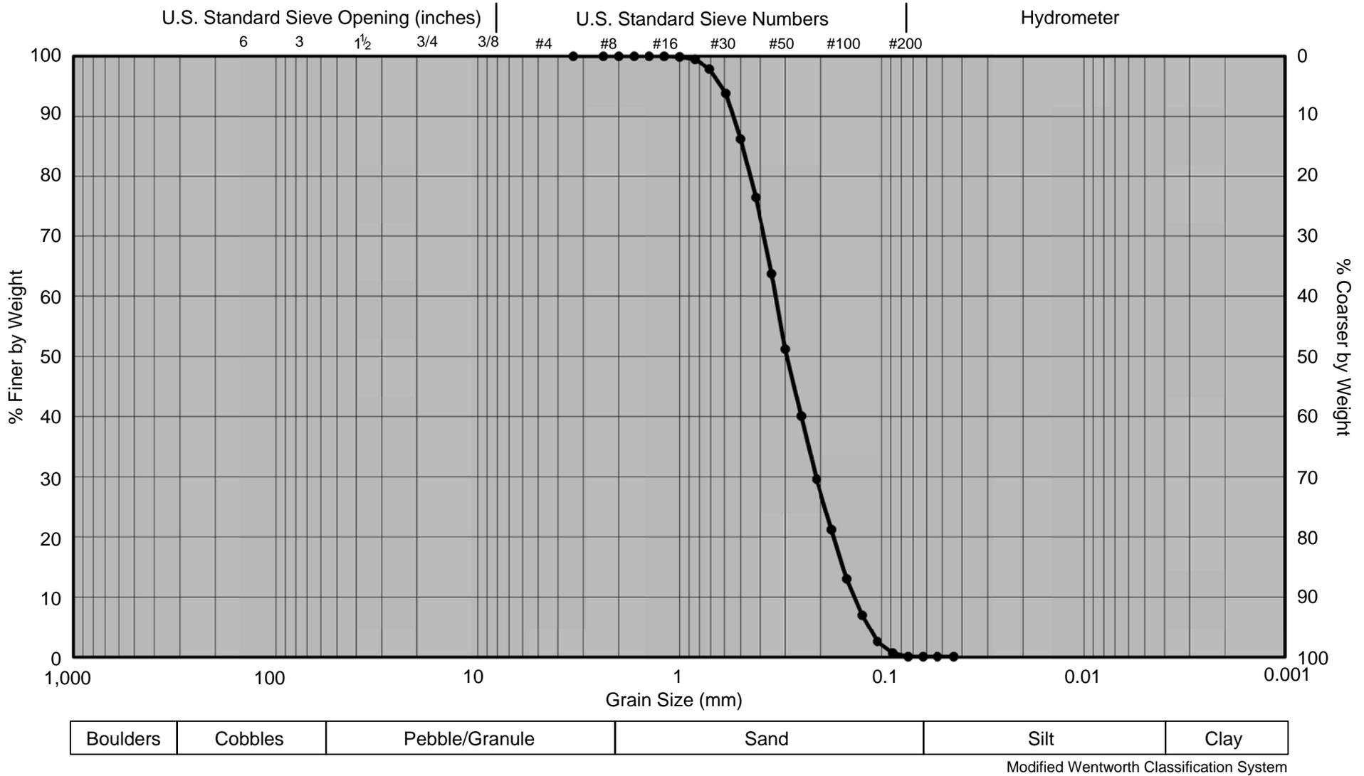
Figure 35. Bulk Sample Grain-Size Distribution Diagram for Sample No. 2 - Qtou.
