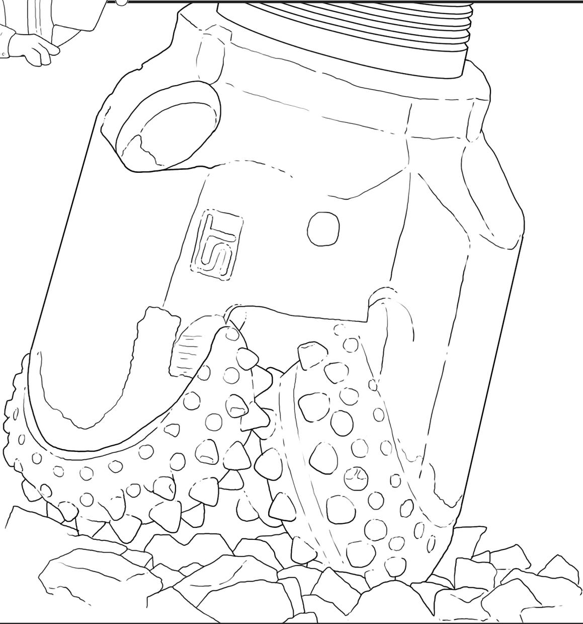
Drilling through solid rock is hard to do, these special drill bits don't cut the rock like a wood cutting drill bit does. Instead of cutting a hole in the rock they actually grind the hole in the rock by breaking off small pieces of rock as they turn the bit.
