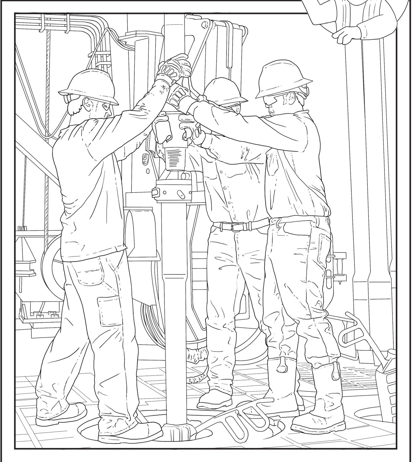
*Over here another rig-hand guides the next piece of drill pipe onto the rig floor.*
