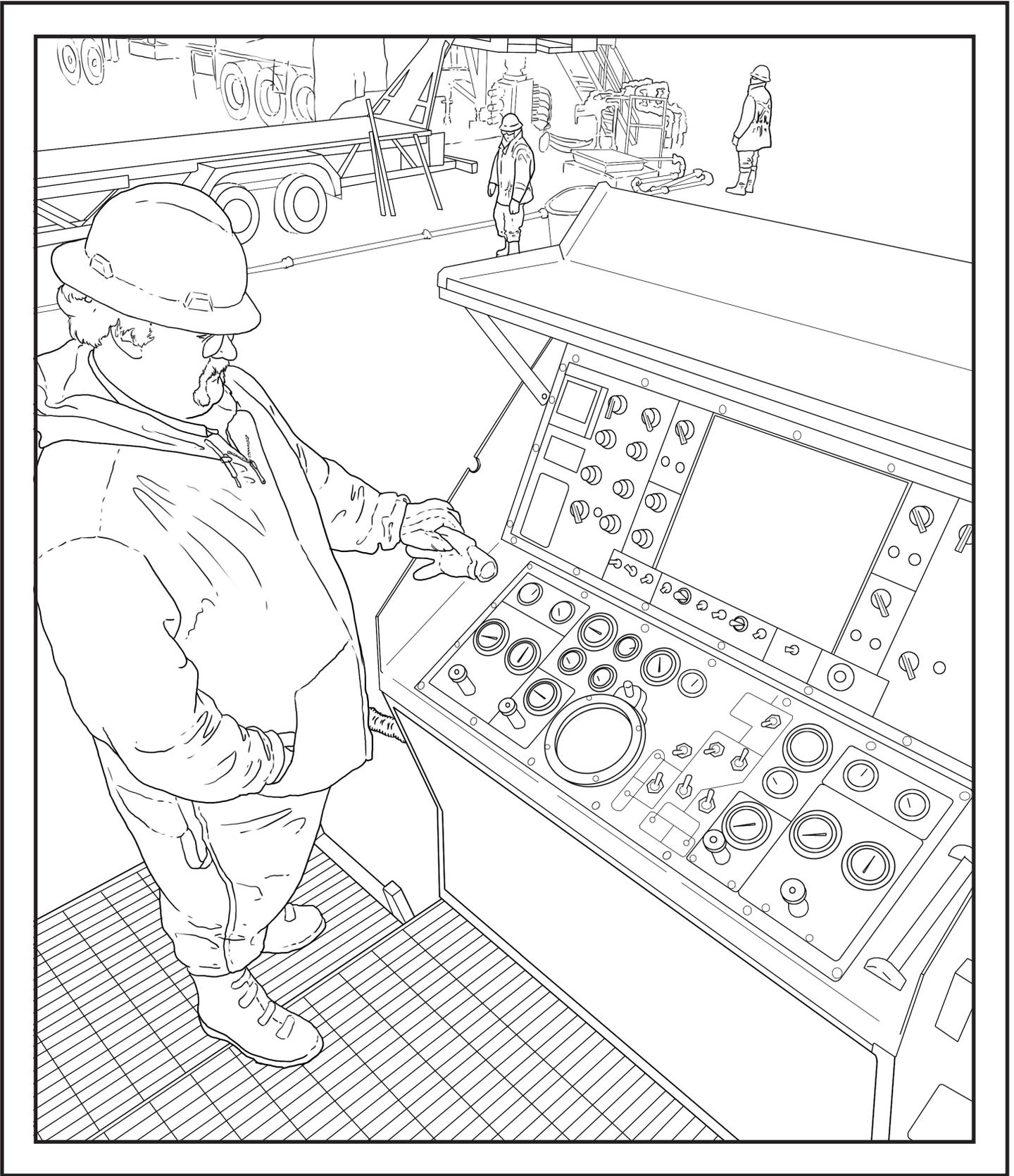
An oil and gas field inspector looks over controls that tell him what is going on down hole during a plugging operation. Once the well has been plugged, surface equipment will be removed and the company will begin the process of returning the land as close as possible to the original condition, through a process called reclamation.
