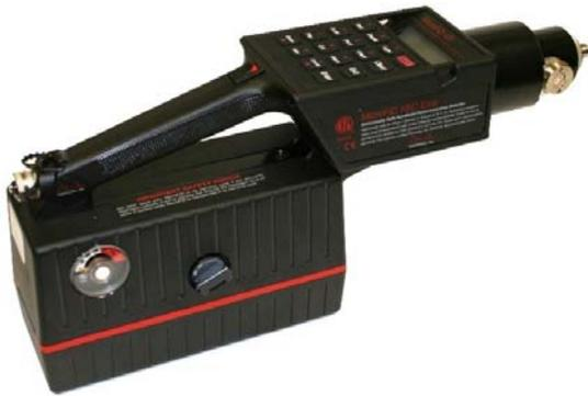
in a high concentration range of 10 ppm to 50,000 ppm with an accuracy of 0.5 ppm within plus or minus 0.5 ppm or plus or minus 10% of the actual C1 concentration when operating in the low (0.5 ppm to 2000 ppm) concentration range. FID instrument precision is plus or minus 0.3 ppm or plus or minus 5% when operating within both the low and high concentration ranges (Photovac, 2007). The instrument response time is effectively immediate.
