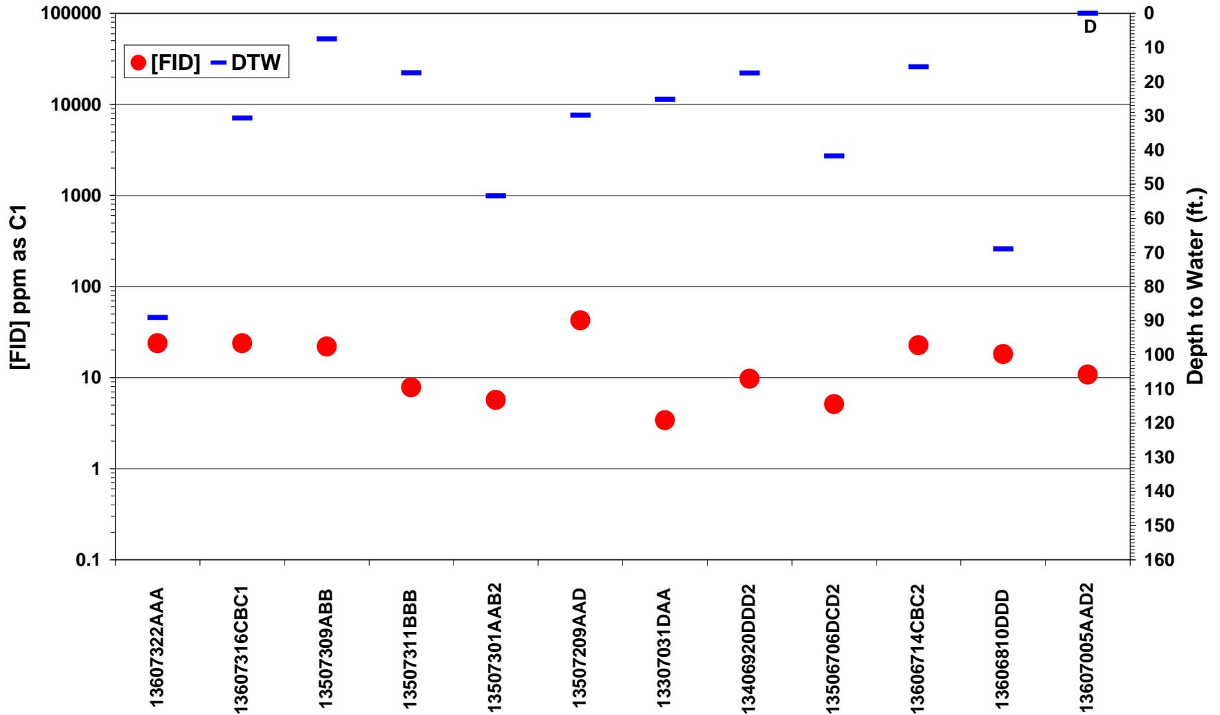
Figure 27. Shallow gas field screening results in Logan County. FID response [FID] in ppm as C1 plotted on the logarithmic scale on the primary y-axis. Depth to water measurements are plotted on the secondary y-axis. Dry wells (D) are highlighted.
