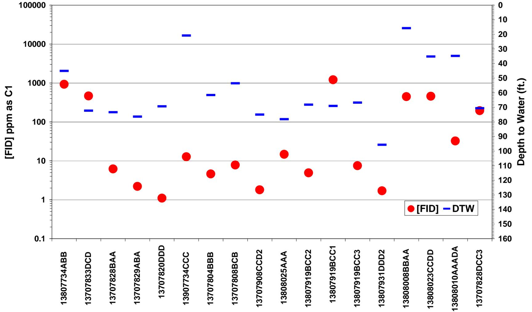
Figure 17. Shallow gas field screening results in Burleigh County. FID response [FID] in ppm as C1 plotted on the logarithmic scale on the primary y-axis. Depth to water measurements are plotted on the secondary y-axis.
