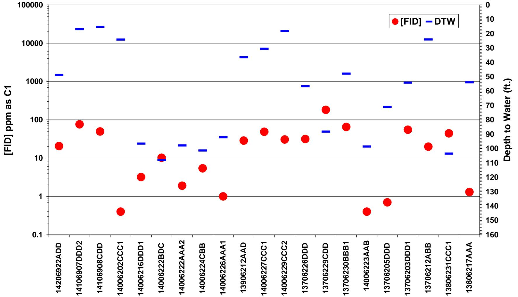
Figure 14. Shallow gas field screening results in Stutsman County. FID response [FID] in ppm as C1 plotted on the logarithmic scale on the primary y-axis. Depth to water measurements are plotted on the secondary y-axis.
