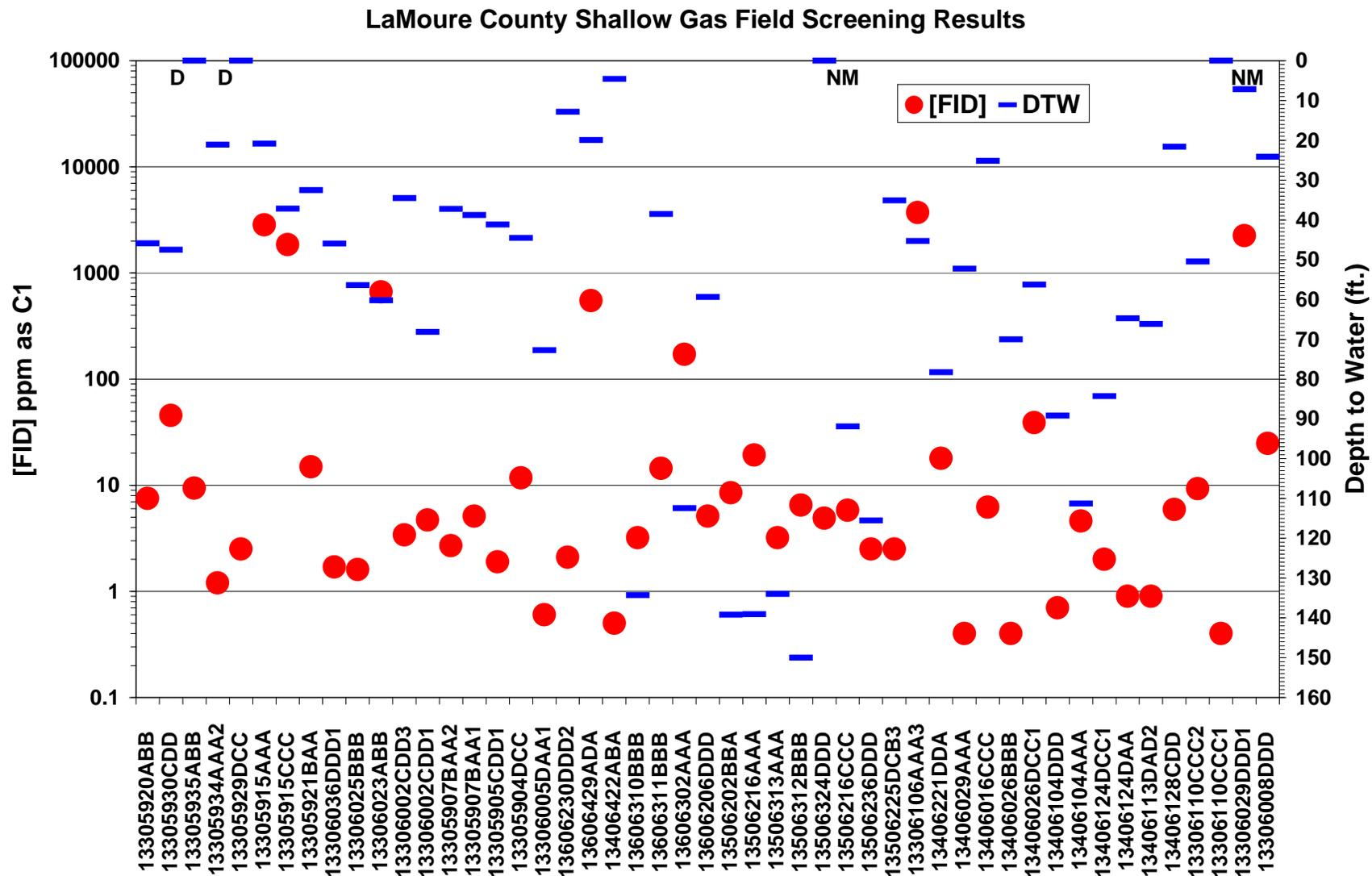
Figure 22. Shallow gas field screening results in LaMoure County. FID response [FID] in ppm as C1 plotted on the logarithmic scale on the primary y-axis. Depth to water measurements are plotted on the secondary y-axis. Wells where a water level was not measured (NM) or were dry (D) are highlighted.
