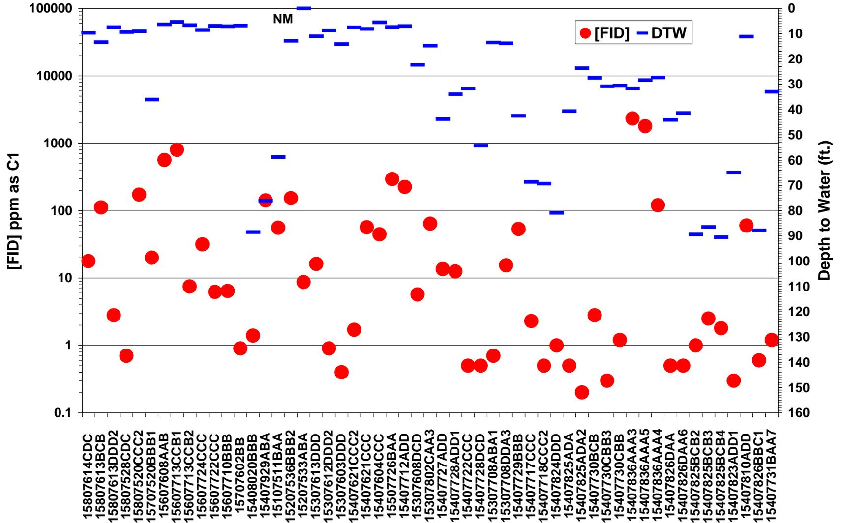
Figure 20. Shallow gas field screening results in McHenry County. FID response [FID] in ppm as C1 plotted on the logarithmic scale on the primary y-axis. Depth to water measurements are plotted on the secondary y-axis.
