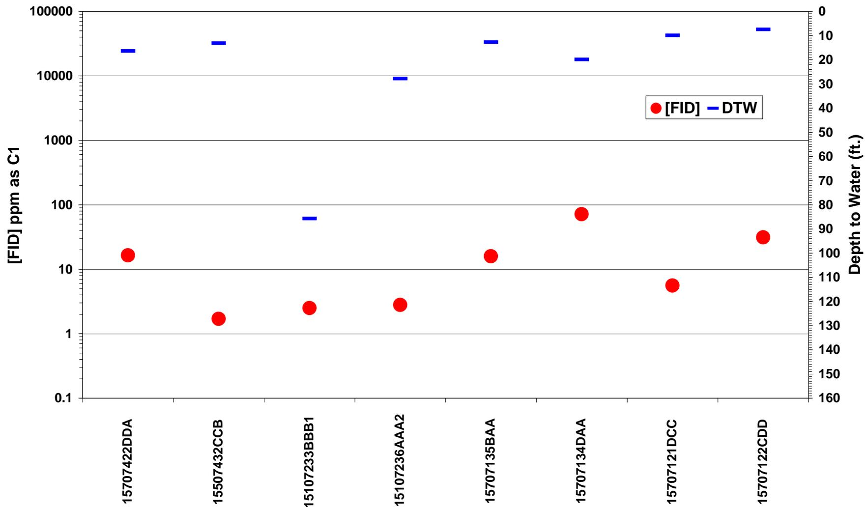
Figure 24. Shallow gas field screening results in Pierce County. FID response [FID] in ppm as C1 plotted on the logarithmic scale on the primary y-axis. Depth to water measurements are plotted on the secondary y-axis.
