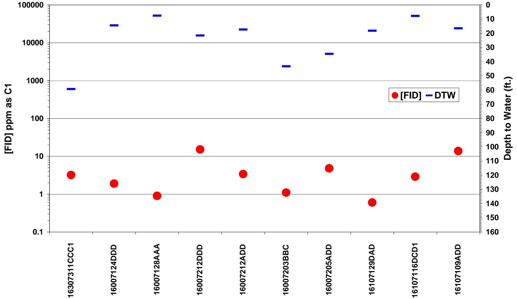
Figure 15. Shallow gas field screening results in Rolette County. FID response [FID] in ppm as C1 plotted on the logarithmic scale on the primary y-axis. Depth to water measurements are plotted on the secondary y-axis.
