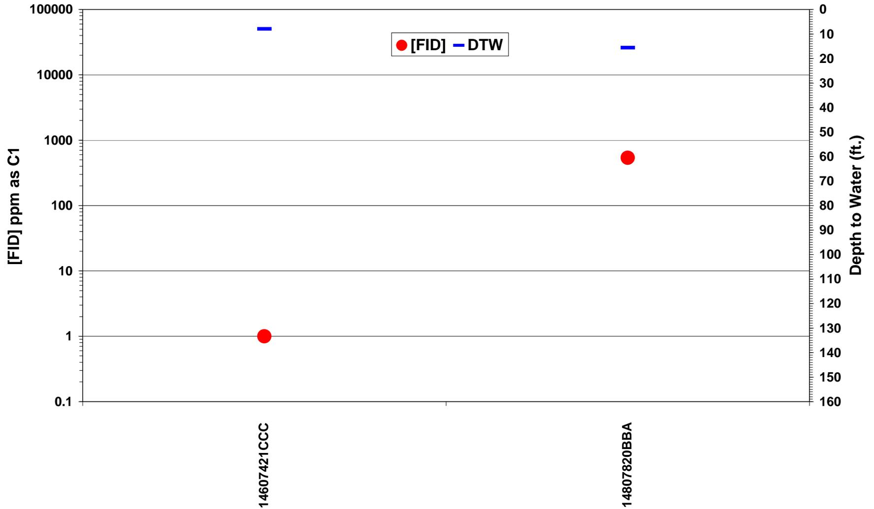
Figure 25. Shallow gas field screening results in Sheridan County. FID response [FID] in ppm as C1 plotted on the logarithmic scale on the primary y-axis. Depth to water measurements are plotted on the secondary y-axis.
