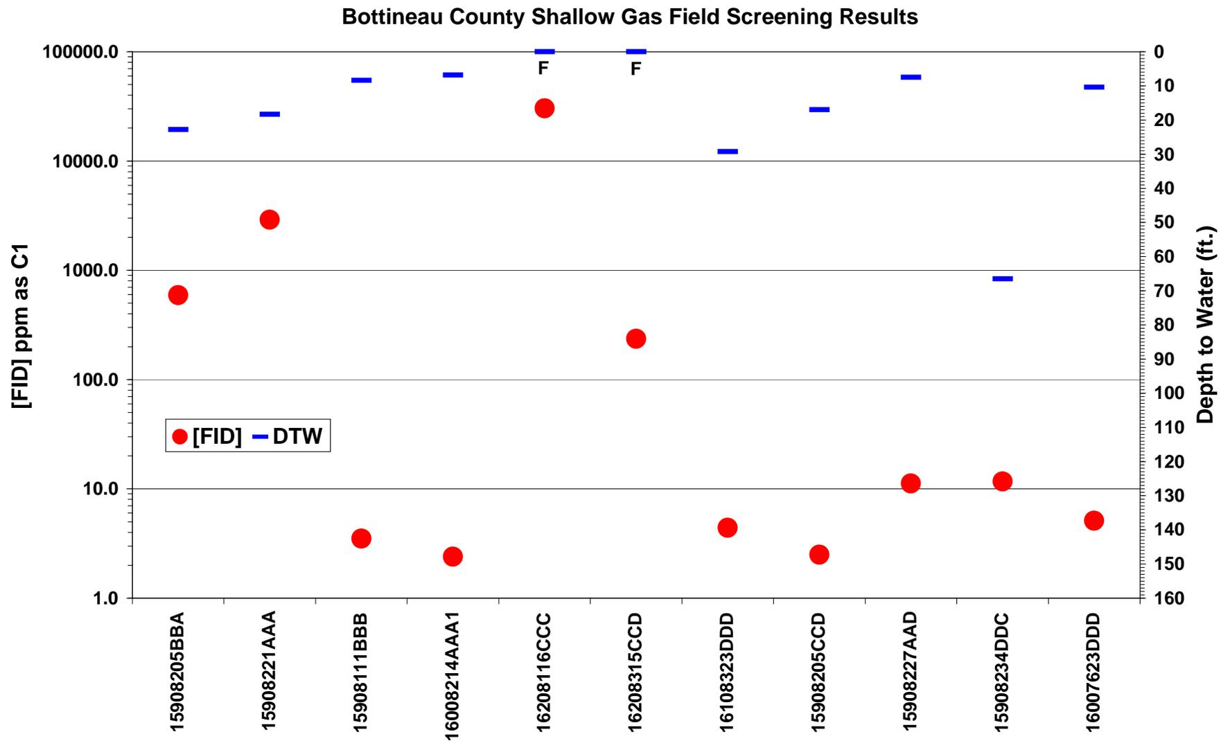
Figure 11. Shallow gas field screening results in Bottineau County. FID response [FID] in ppm as C1 plotted on the logarithmic scale on the primary y-axis. Depth to water measurements are plotted on the secondary y-axis. Flowing wells (F) are highlighted.
