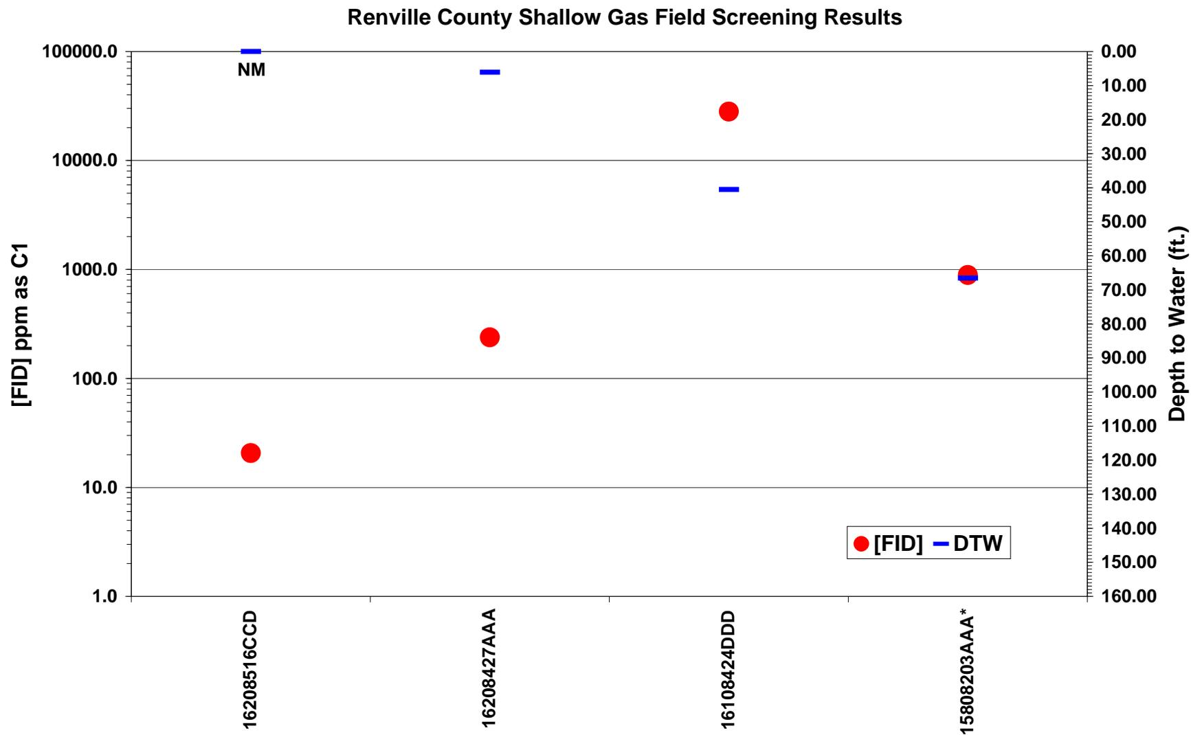
Figure 12. Shallow gas field screening results in Renville County. FID response [FID] in ppm as C1 is plotted on the logarithmic scale on the primary y-axis. Depth to water measurements are plotted on the secondary y-axis. \*Collected on June 26, 2007.
