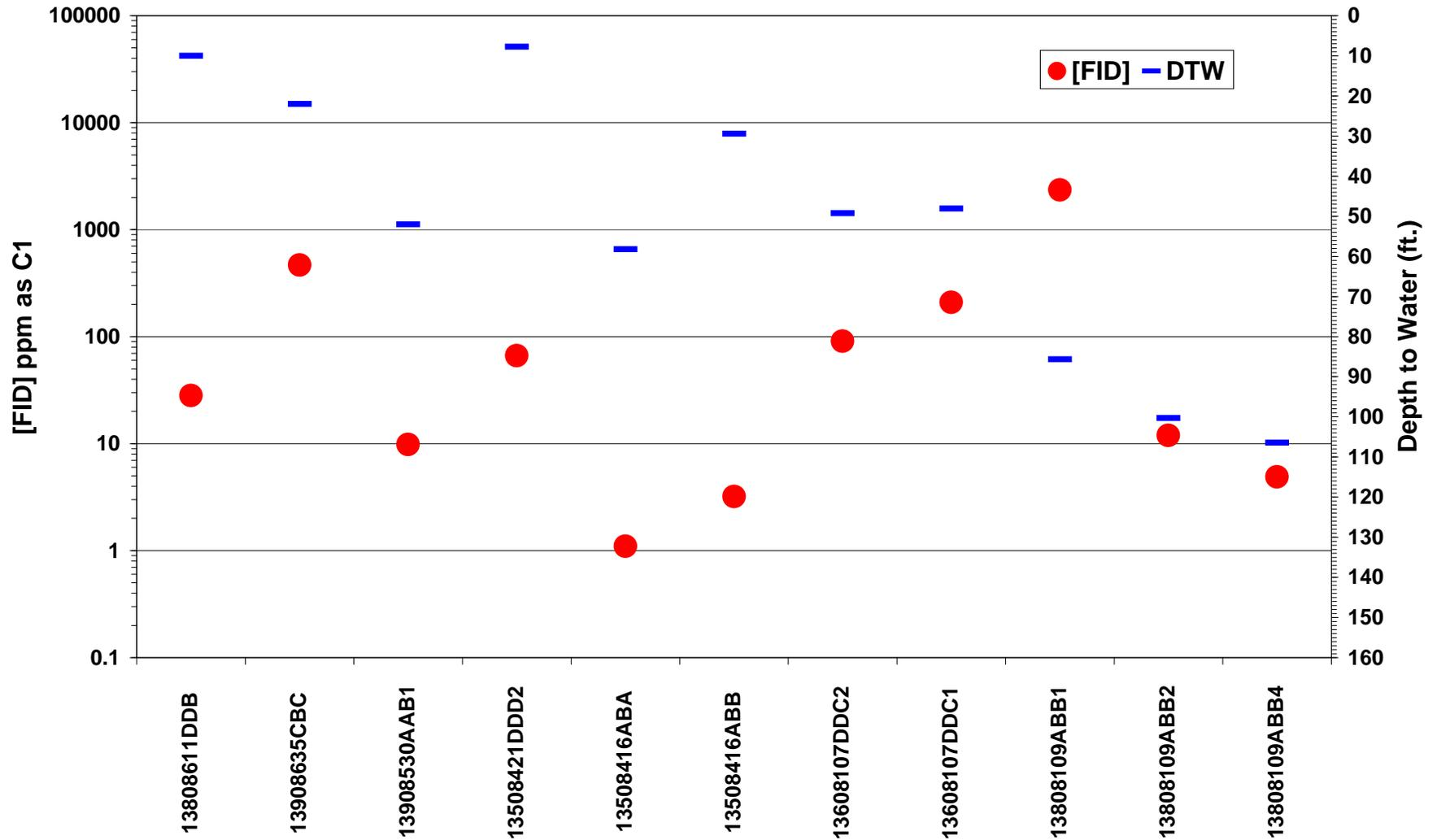
Figure 23. Shallow gas field screening results in Morton County. FID response [FID] in ppm as C1 plotted on the logarithmic scale on the primary y-axis. Depth to water measurements are plotted on the secondary y-axis.
