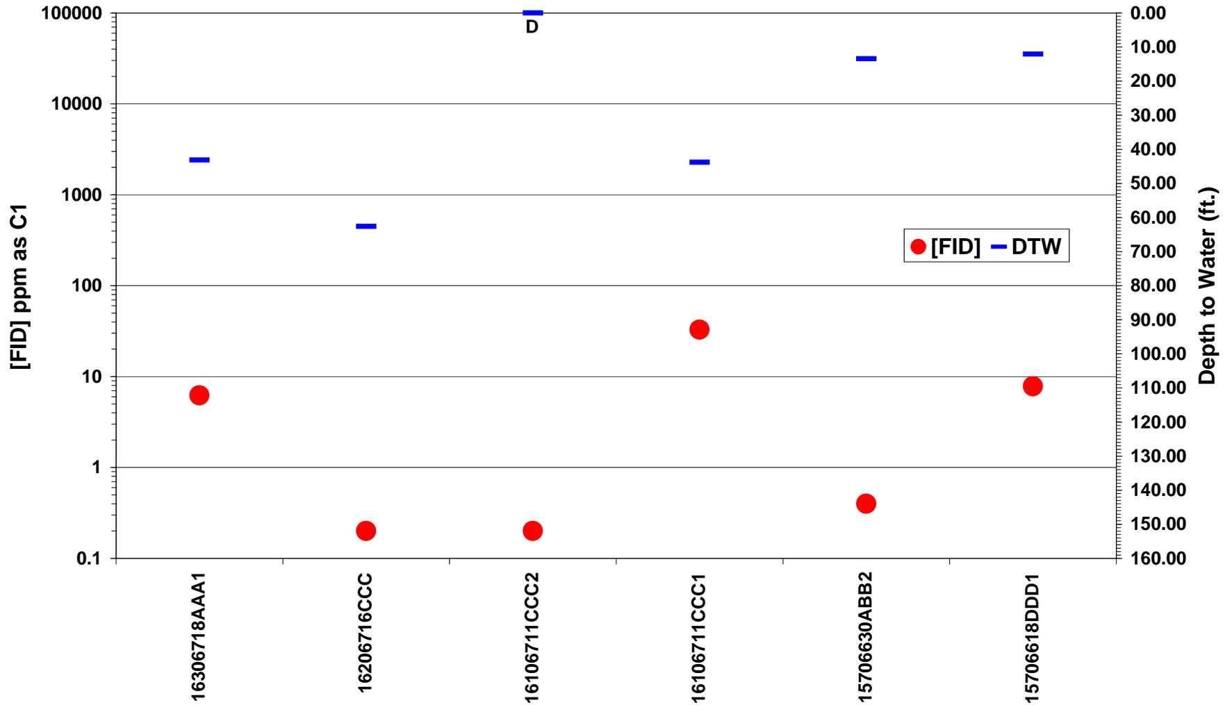
Figure 16. Shallow gas field screening results in Towner County. FID response [FID] in ppm as C1 plotted on the logarithmic scale on the primary y-axis. Depth to water measurements are plotted on the secondary y-axis. Well with no measurable water level (D) highlighted.
