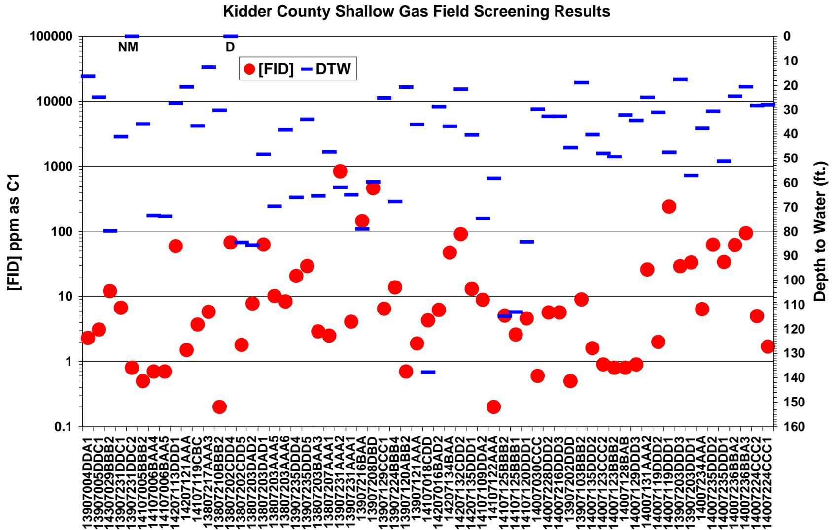
Figure 18. Shallow gas field screening results in Kidder County. FID response [FID] in ppm as C1 plotted on the logarithmic scale on the primary y-axis. Depth to water measurements are plotted on the secondary y-axis. Wells where a water level was not measured (NM) or were dry (DRY) are highlighted.
