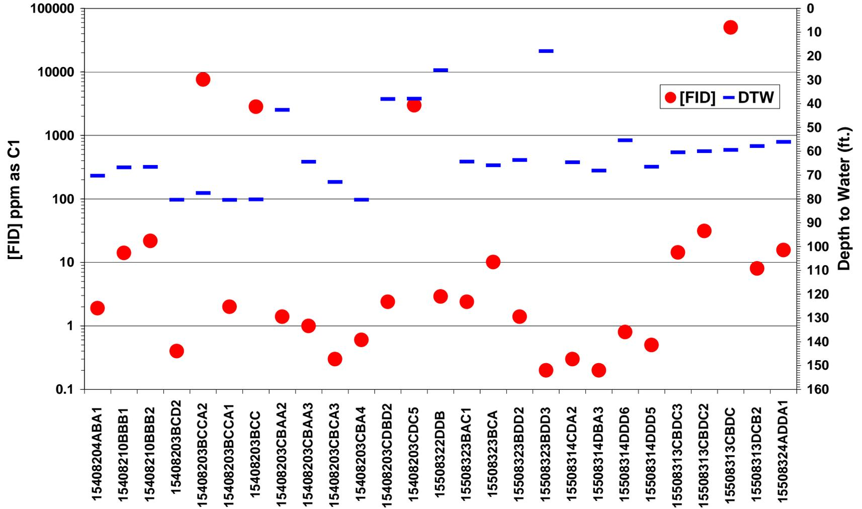
Figure 19. Shallow gas field screening results in Ward County. FID response [FID] in ppm as C1 plotted on the logarithmic scale on the primary y-axis. Depth to water measurements are plotted on the secondary y-axis.
