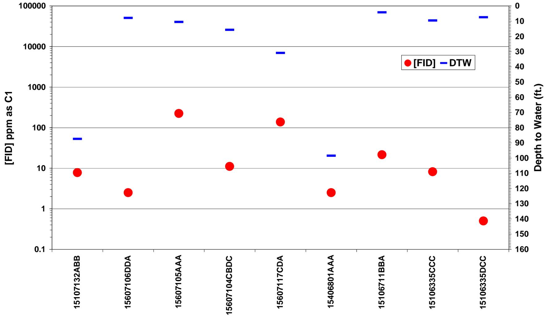
Figure 26. Shallow gas field screening results in Benson County. FID response [FID] in ppm as C1 plotted on the logarithmic scale on the primary y-axis. Depth to water measurements are plotted on the secondary y-axis.
