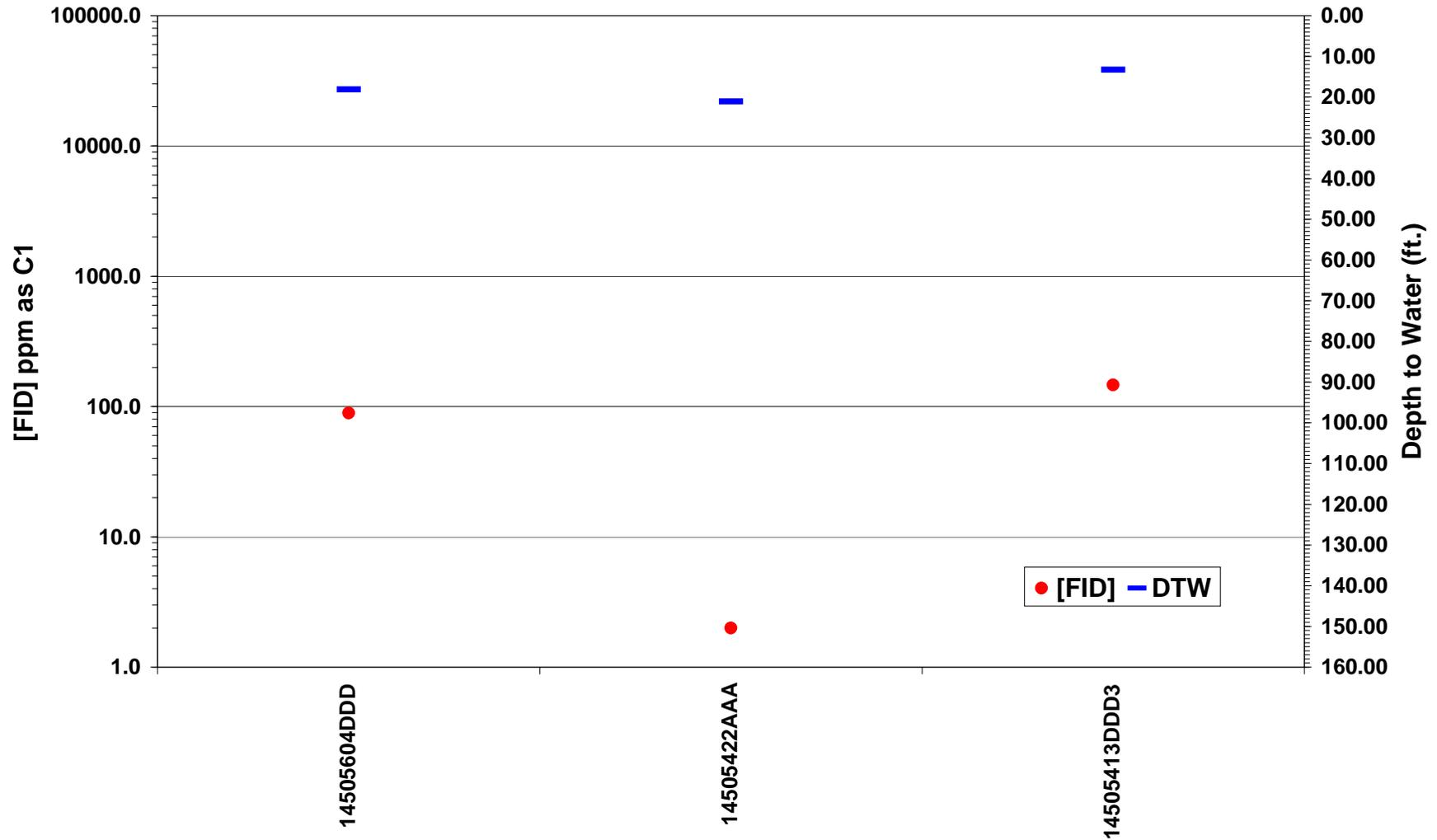
Figure 10. Shallow gas field screening results in Steele County. FID response [FID] in ppm as C1 is plotted on the logarithmic scale on the primary y-axis. Depth to water measurements are plotted on the secondary y-axis.
