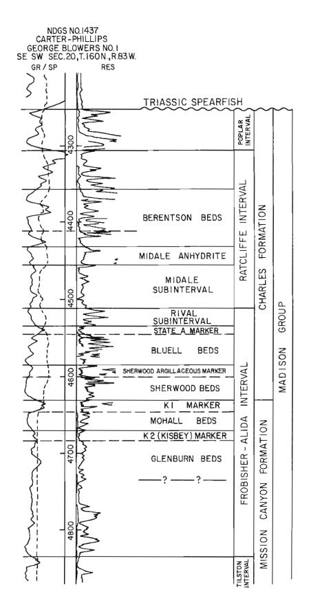
Figure 2. A typical log showing the subdivisions of the Ratcliffe and Frobisher-Alida intervals used in this paper.
