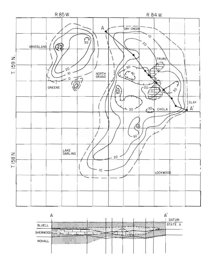
Figure 4. Isopach map of the argillaceous anhydrite within the Bluell beds and associated carbonate thickenings.
