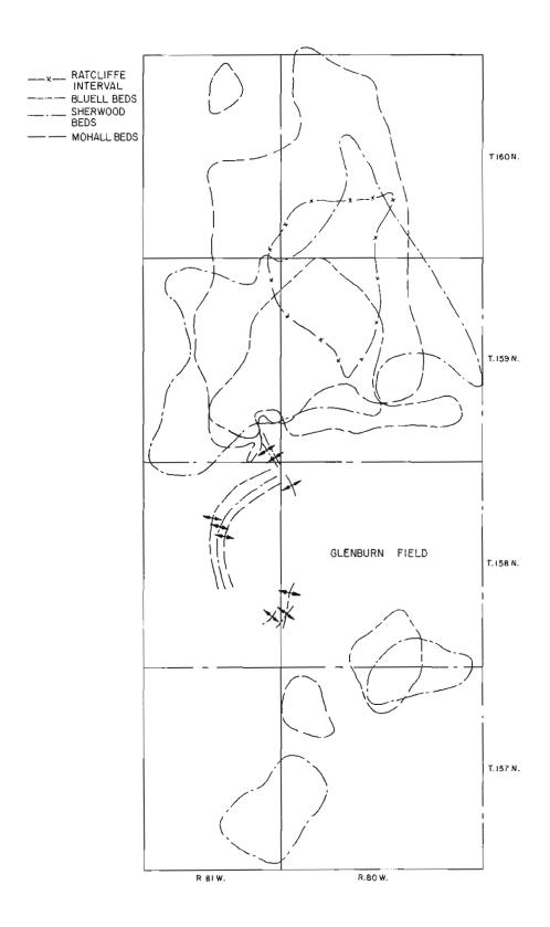
Figure 6. Map indicating the distribution of areas of thicker sediments north and south of Glenburn Field, including the distribution of hinge lines of the informal units for the Glenburn Field.
