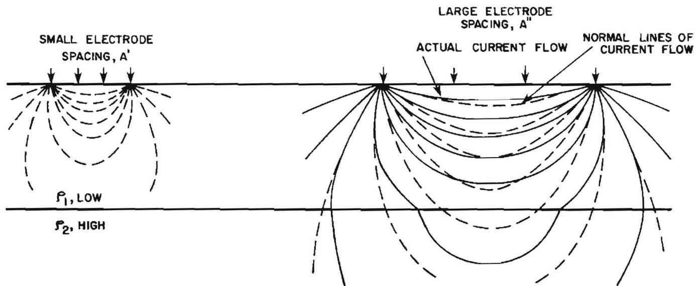
Figure 3. Influence of a layer of high resistivity at depth on the lines of current flow as the vertical electrode sounding (VES) is expanded from small electrode spacings (left) to large electrode spacings (right). Current flow tends to become concentrated in the more conductive layer and therefore higher apparent resistivity readings are obtained. (From Soiltest, 1968.)
