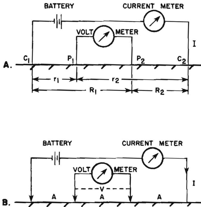
Figure 2. A. Configuration of the four-electrode array used in earth resistivity work. Current is passed through electrodes  $C_1$  and  $C_2$  and potential difference readings are made between electrodes  $P_1$  and  $P_2$ . Distances below are used in derivation of formulas for apparent resistivity.
