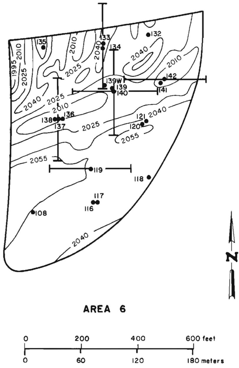
Figure 8. Precontouring topography (elevations in feet) of area 6 at the Center Mine. Piezometer locations shown as dots and resistivity surveys shown as heavy lines.
