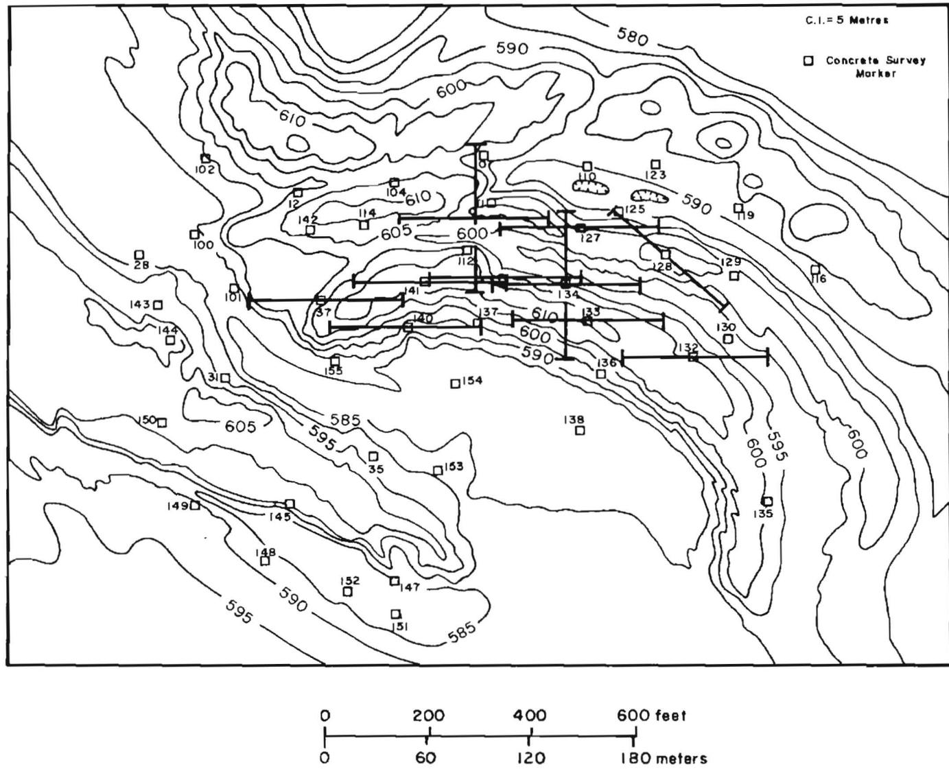
Figure 4. USBM spoils study area at the Indian Head Mine. Contours indicate topography of spoils prior to reclamation. Resistivity surveys are shown by heavy lines and identified by concrete markers located along survey traverse (see app. IIB).
