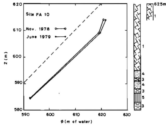
Figure 7. Measured hydraulic profiles through the saturated zone at eight piezometer nests in the Falkirk study area, where 1 is pebble-loam, 2 is sand and gravel, 3 is silty clay to clayey silt, 4 is silty fine to medium sand, and 5 is lignite. The eight graphs comprising this figure are on pages 13 through 17.
