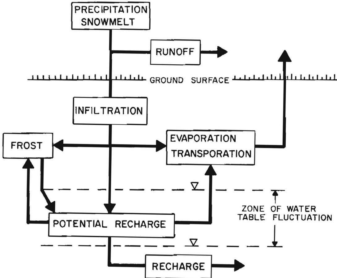
Figure 4. Potential paths of water movement from the ground surface to the water table.
