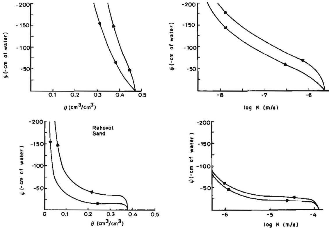
Figure 5. Measured values of hydraulic conductivity ( $K(\psi)$ ) and soil moisture ( $\theta(\psi)$ ) for Grenville silt loam and Rehovot sand (after Freeze, 1969).
