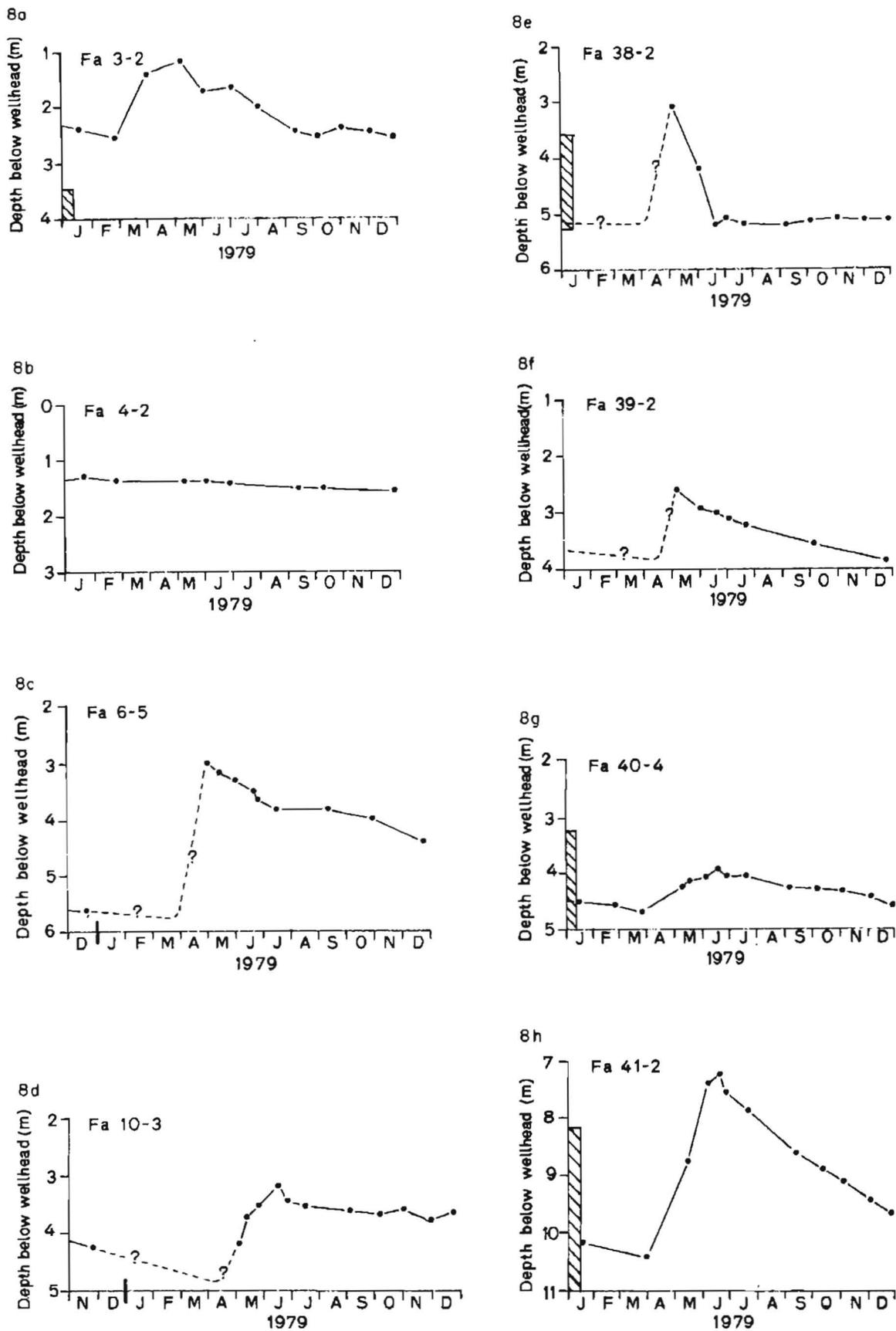
Figure 8. Hydrographs from water-table observation wells and shallow piezometers. The thirty-three graphs comprising this figure are on pages 22 through 25.
