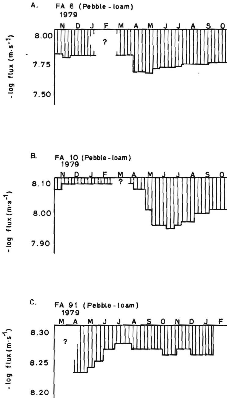
Figure 10. Vertical flux of water in the saturated zone at six plezometer nests in the Falkirk study area. The six graphs comprising this figure are on pages 32 and 33.
