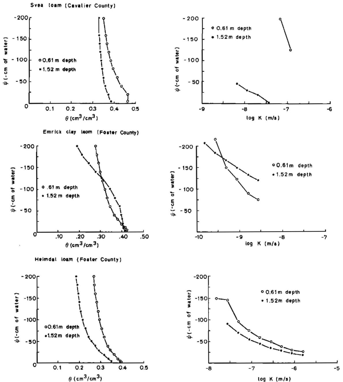
Figure 6. Measured values of hydraulic conductivity ( $K(\psi)$ ) and soil moisture ( $\theta(\psi)$ ) of three loamy soils from eastern North Dakota (after Cassel, 1974).
