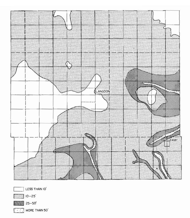
Fig. 4. Thickness of the Coleharbor Formation which overlies the Pierre Shale in the Langdon area.
