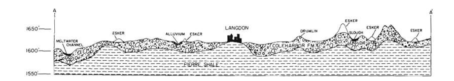
Fig. 3. Generalized northeast-southwest (A-A') cross section showing the Coleharber Formation and the top of the Pierre Shale.
