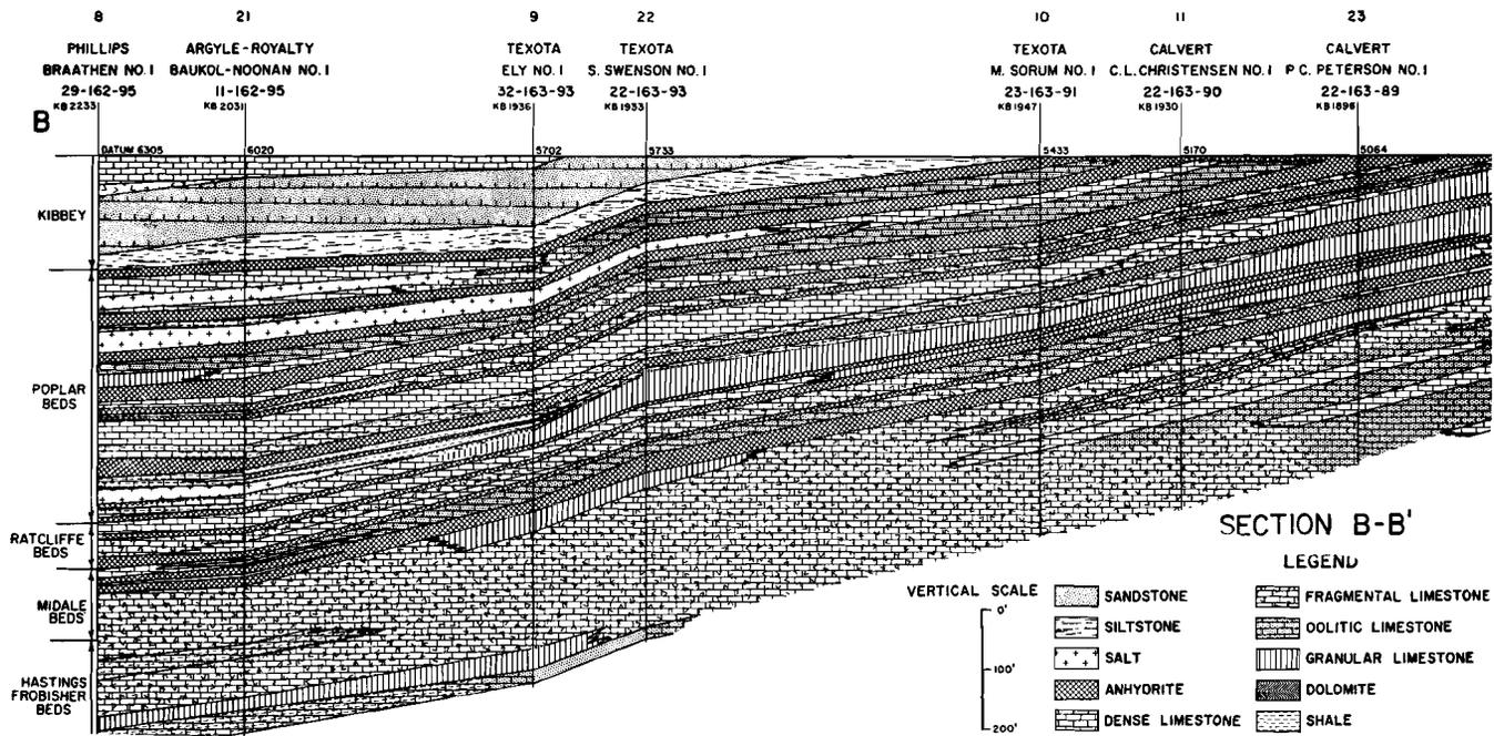
FIGURE 3—This cross-section B-B's is a geologic east-west cross-section extending from Phillips Petroleum Company's Braathen 1, Sec. 29-162-95, to Cardinal Drilling Company—U.C.L.I. 1, Sec. 1-163-81. Datum for this cross-section is the top
