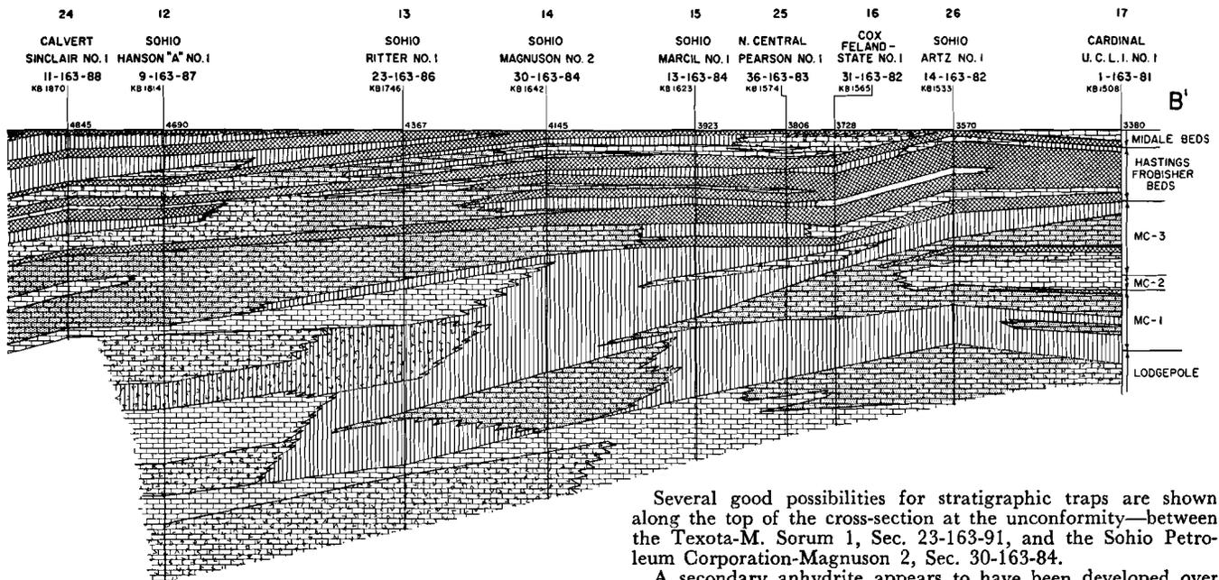
of the Kibbey limestone as far east as the limestone extends, and from that point eastward the post-Mississippian unconformity is used for a datum.
