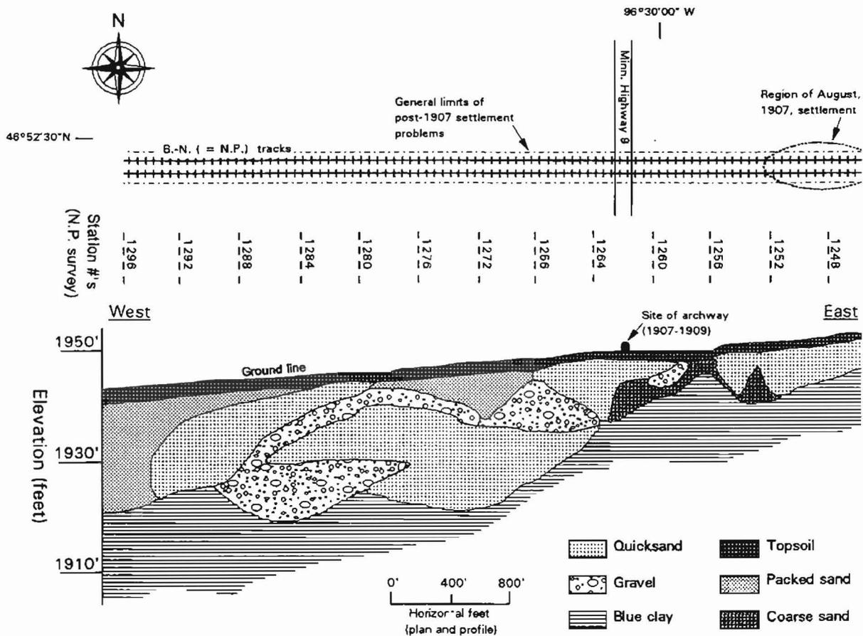
**Figure 1.** Plan view and geologic cross-section of Stockwood Fill in the region of the present-day Minnesota Highway 9 underpass. Cross-section is re-sketched from soundings profile of S.A. McCoy (November 1, 1909).
