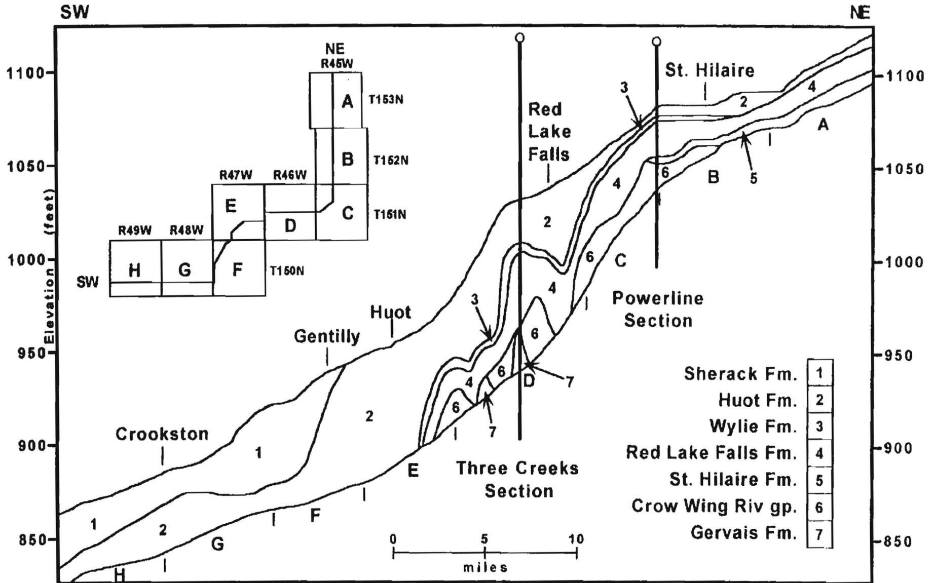
Figure 13. Generalized cross section along the Red Lake River in the Red Lake Falls, Minnesota area (modified from Harris and others, 1974).
