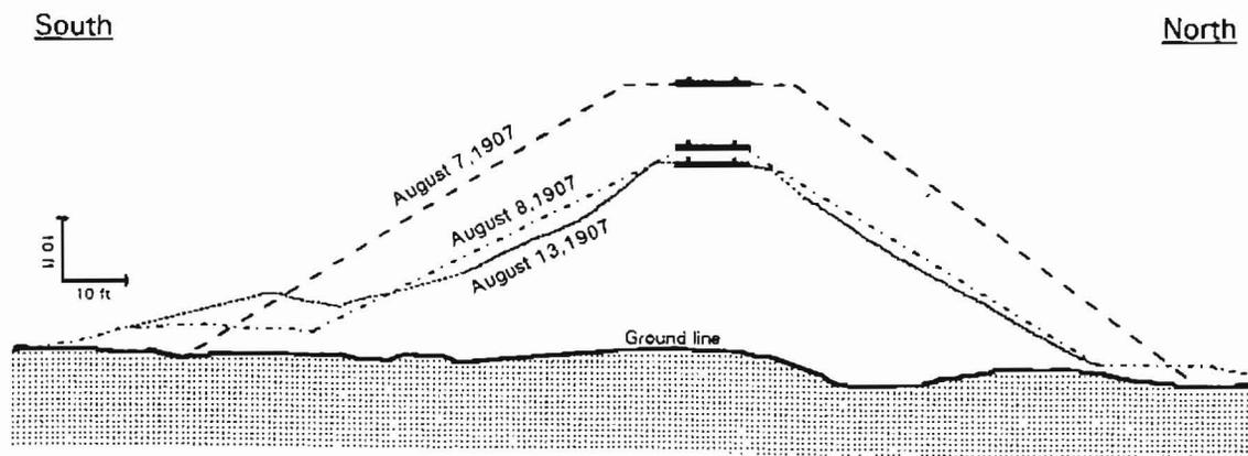
**Figure 4.** Profile changes at station #1245, Stockwood Fill, August 7 - 13, 1907. (Re-sketched from an N.P. profile, probably dating to August 13, 1907).
