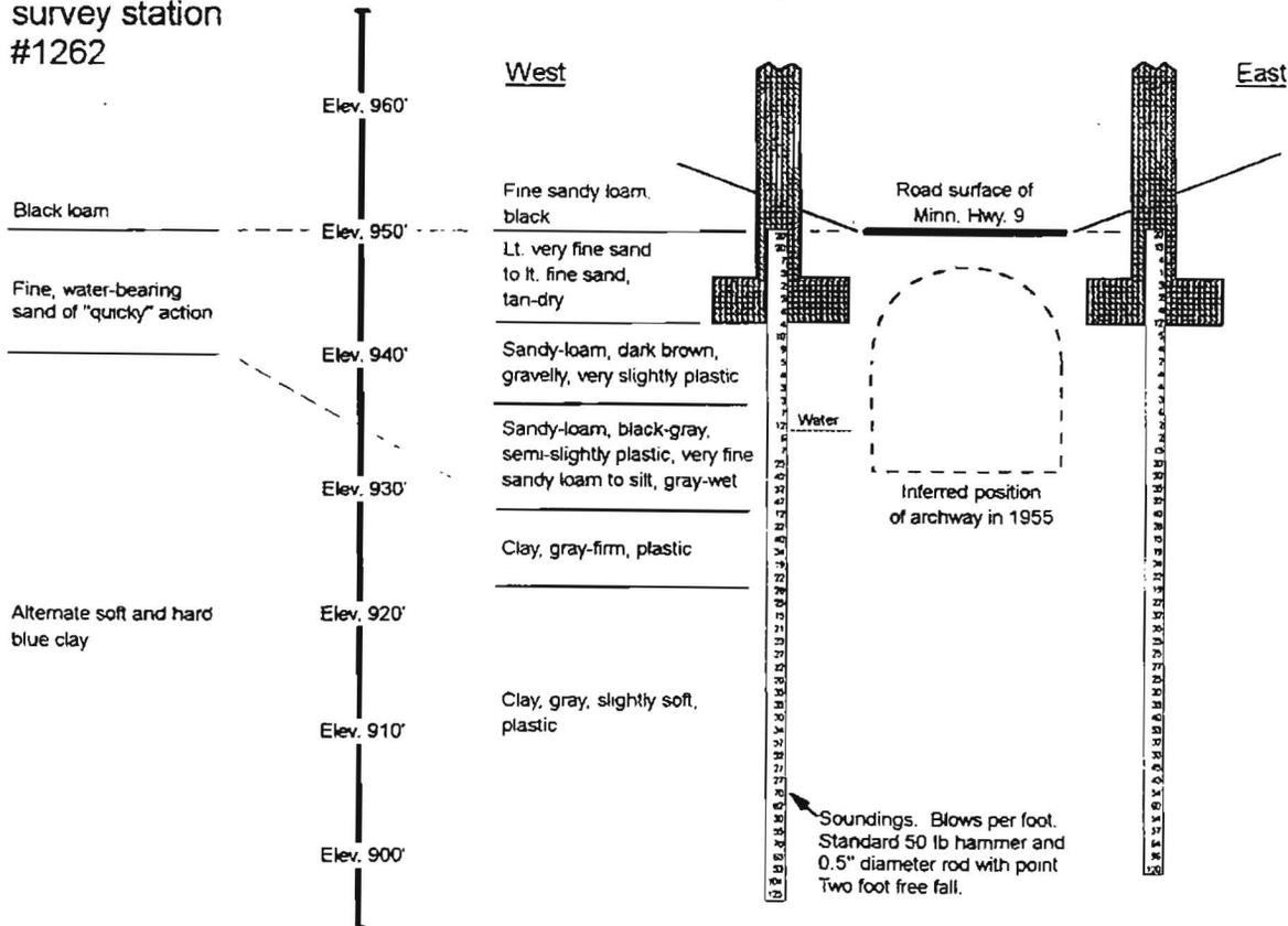
Figure 6. Comparison of soil test profiles in the region of Stockwood Fill station #1262 (data from S.A. McCoy, 1907, and Minnesota Dept. of Highways, 1955).
