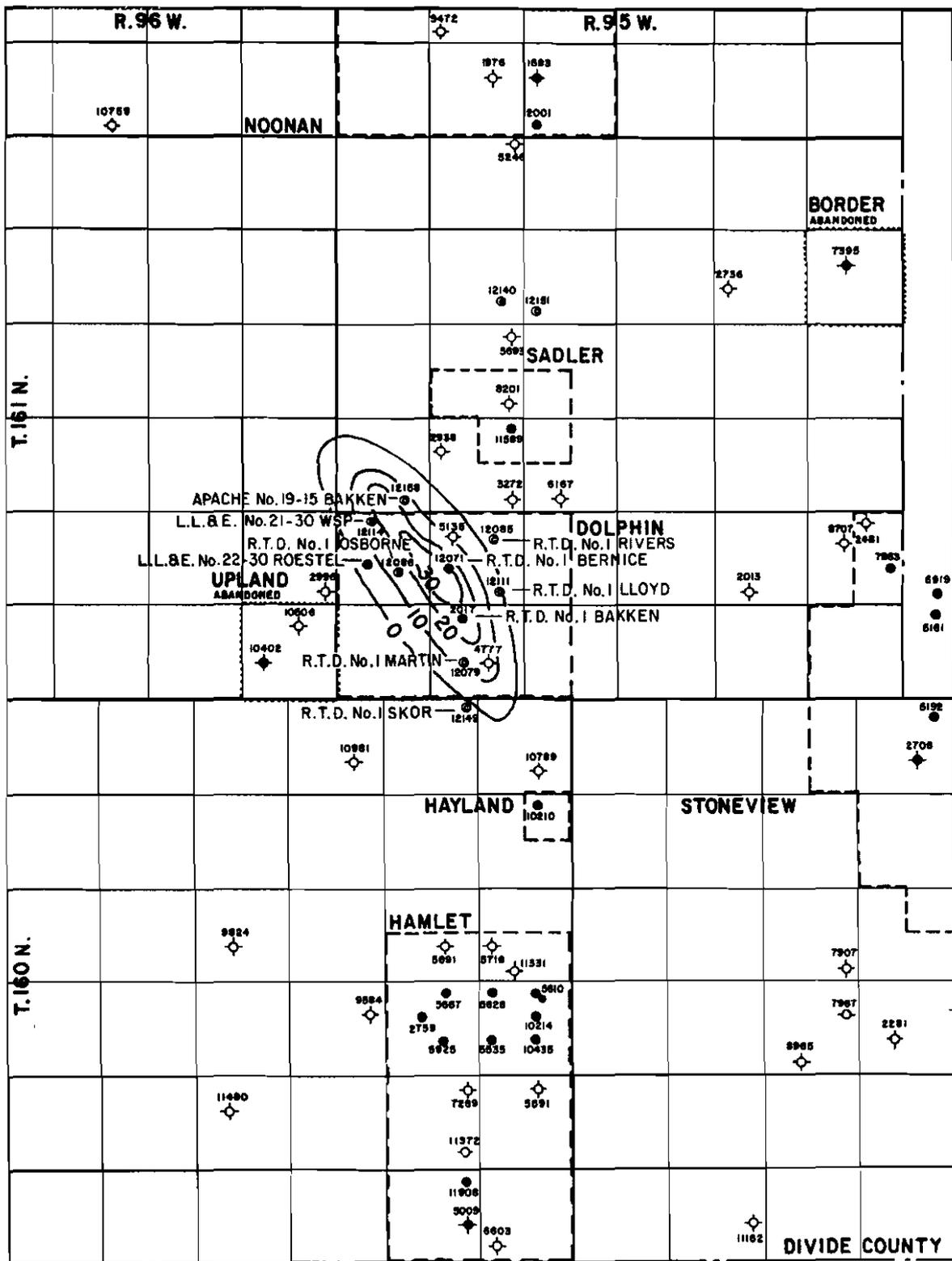
Figure 4. Net feet of greater than 6% crossplot porosity, Dolphin field, Divide County, North Dakota. Also shown are the names and locations of field tests. Contour interval = 10 feet.
